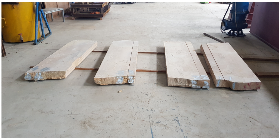
Figure 2.8: The first batch of sandstone samples used for the cutting experiments
