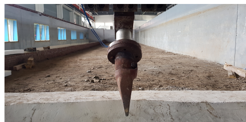
(b) Pick point mounted on pressure sensor
