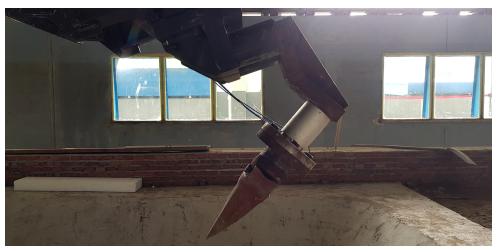
(a) Pressure sensor mounted on transition piece
