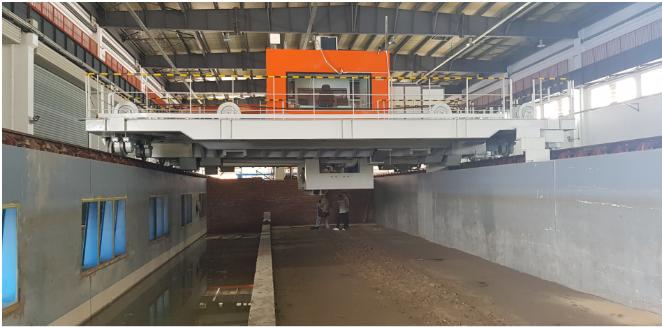
Figure 2.3: Movable platform, as seen from the water flume
