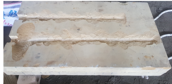
(b) Cutting profile in rock sample after experiment
