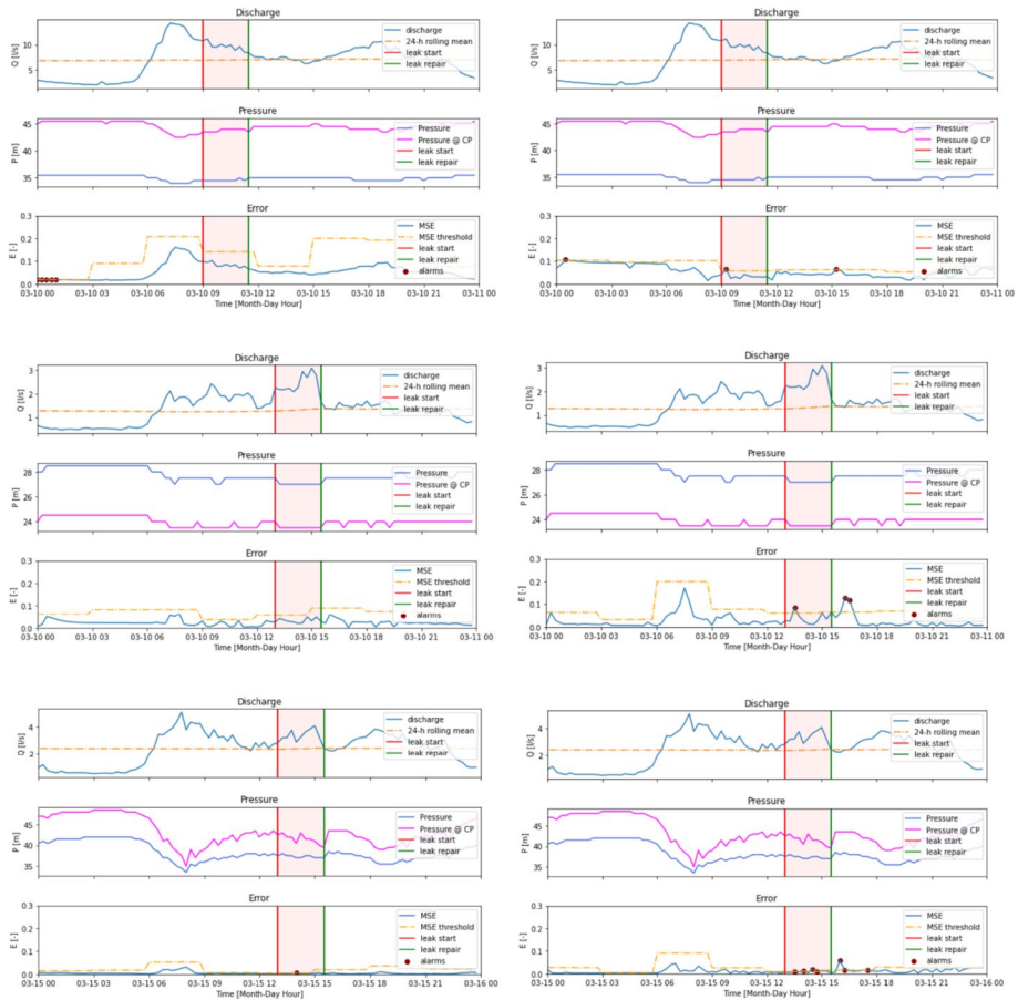
Fig. 2 Fire hydrant bursts in DMAs Beta (top), Delta (middle) and Zeta (bottom). Left sub-figures are for Scenario A. Right sub-figures are for Scenario C. Top row is for the discharge at the inflow of the DMA.. Middle row is for the pressure at the inflow of the DMA and the critical point. Lower row is for the MSE (error), the error threshold, the burst start and repair time and the raised alarms
