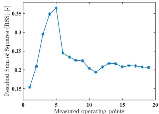
Figure 14 Residual sum of squares of the cylinder model at the calibrating operating points dataset
