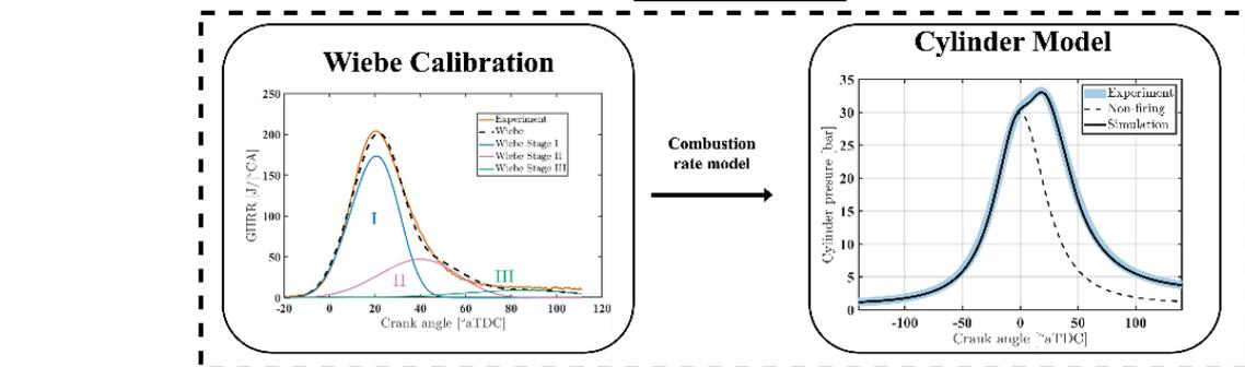
Figure 3 Methodology for the development and calibration of the cylindrical model based on Wiebe functions
