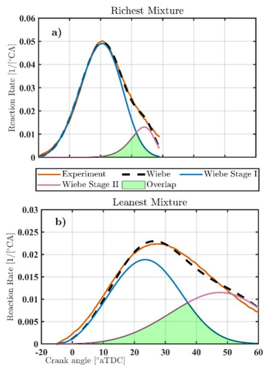
Figure 10 Overlapping of Stage I and II at the richest and leanest mixtures
