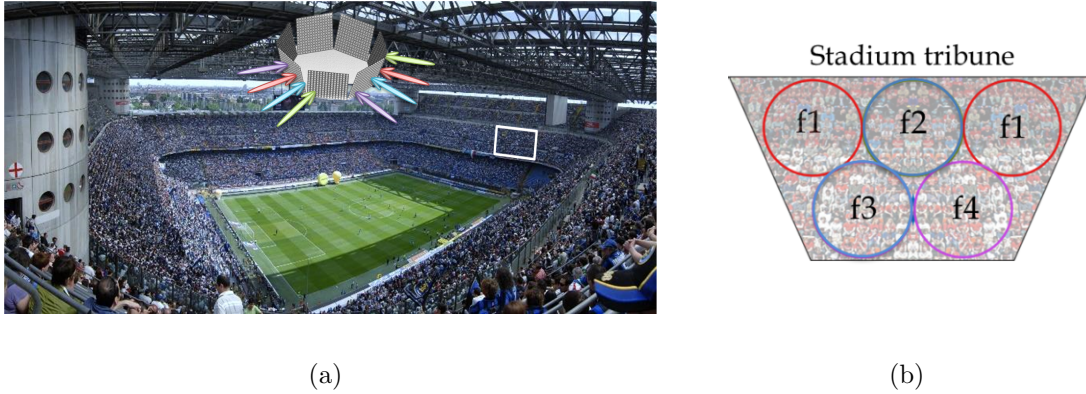
Figure 1.5: a) Football stadium with central base station, generating multiple, fixed beams to cover the full tribune. b) View of part of the stadium tribune with different cells, with an FDMA/SDMA scheme using 4 frequencies.
