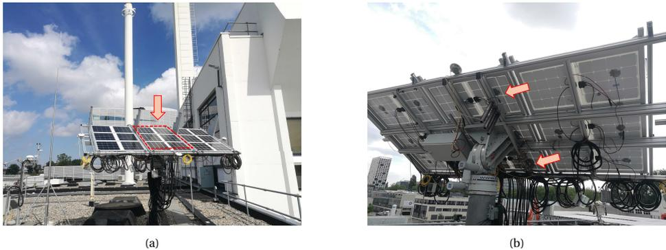
Figure 2.7: (a) Photovoltaic mini modules connected in series and used for the validation of the thermal model (b) Arrows indicating the placement of the thermocouples at the backside of two mini modules.
