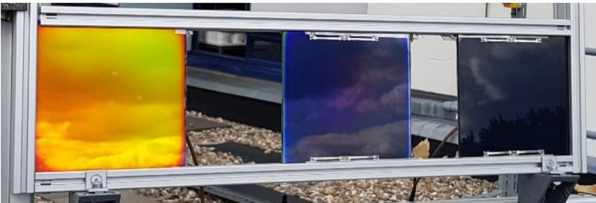
Figure 4.23: Temperature measurements of a colored mini module (Orange, left), a mini module with an experimental filter (middle, outside of the scope of this work) and a standard mini module (right)..
