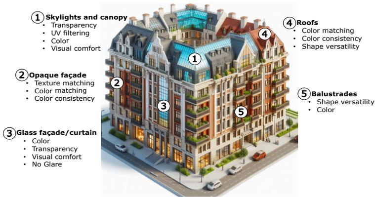
Figure 1.1: Different integration applications within the building environment. 1 Canopy or skylight. 2 Opaque facade. 3 Glass facade / glass curtain. 4 Roofs. 5 Balustrades or external devices. Each application has its particular technical challenges. Image generated via Microsoft Designer: Image creator (Dall-E3 engine)
