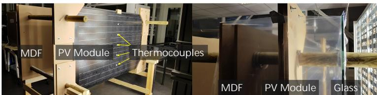
Figure 7.5: The built setup was built according to the physical properties of the PV module used. To the left, the set up without the front glass. The thermocouples were installed in the geometrical middle of the setup, as it is also shown in 7.6. To the right, the full setup with front glass and the plastic side coverage sheets.
