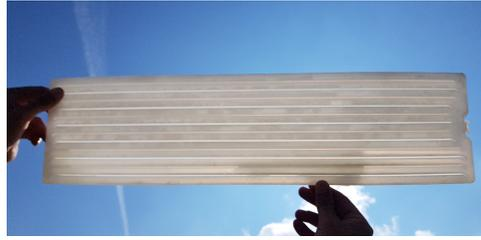
Figure 6.2: Selected Phase change material (PCM) encapsulated in a crystal storage panel made of high-density polyethylene. The panel is divided into 6 sections to avoid mixture separation
