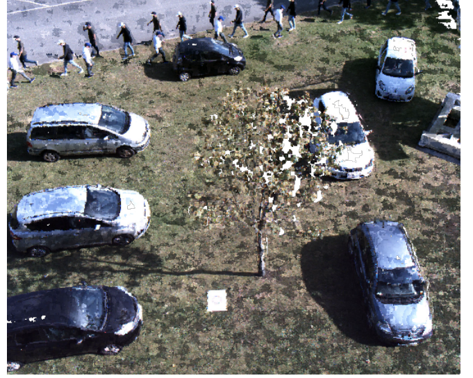
Fig. 17. Real-world Dataset. Screenshot of an overlay of 9 stereo pointclouds. Static cars, the central tree and trajectories followed by the three walking persons can be identified.
