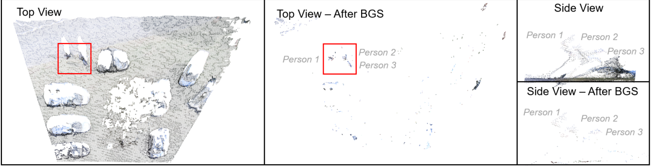
Fig. 16. Background Subtraction (BGS) result on the real-world dataset. The two images for top and side view show the stereo pointcloud before and after BGS based on a 5 component GMM is performed.
