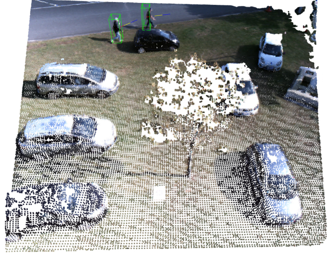
Fig. 1. Output visualisation of the MOSES pipeline. 3D stereo reconstruction of a real-world dataset. Object detections are shown in green and t+1, t+2, t+3 object motion estimates in red, yellow, and blue.
