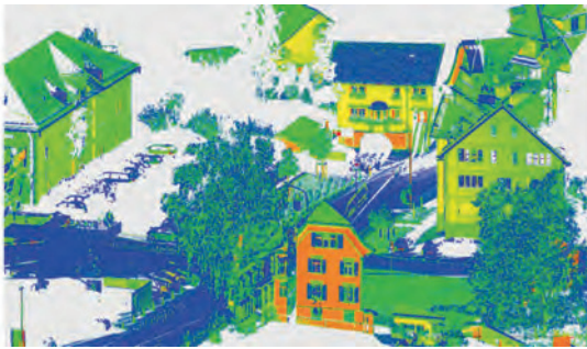
▲ Figure 5, Point cloud of an urban scene in the Semantic3d.net benchmark dataset, intensity coloured.
