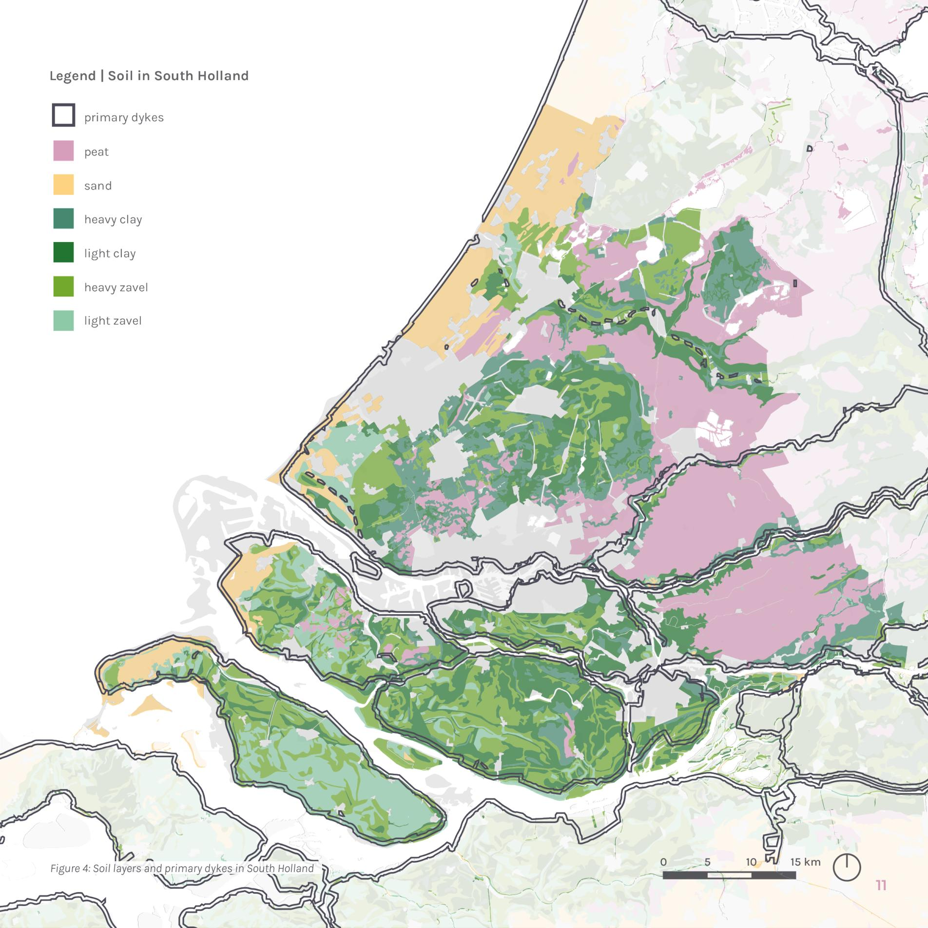
Figure 4: Soil layers and primary dykes in South Holland
