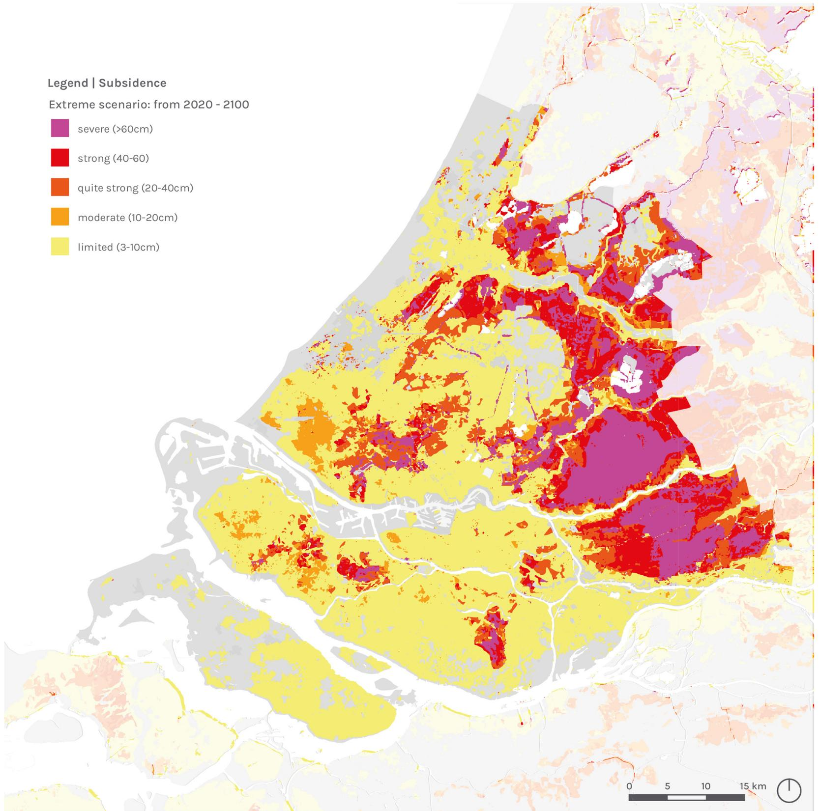
Figure 12: Amount of subsidence between 2020 to 2100
