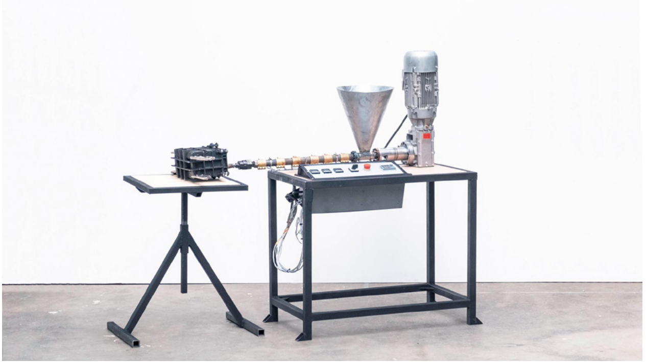
Figure 8 (above) The Extrusion Pro is an open-source design from Precious Plastic that can extrude recycled plastic into a mould. Precious plastic has designed a range of open-source machinery for processing recycled plastic that can be built from widely available materials, making this a prime example of Convivial Materialisation. Image by Precious Plastics (2025), licensed under CC BY 4.0.
