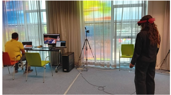
Figure 2: System setup at the museum, showing the client participant (curator) wearing a head-mounted display and being captured by cameras for real-time pointcloud representation.
