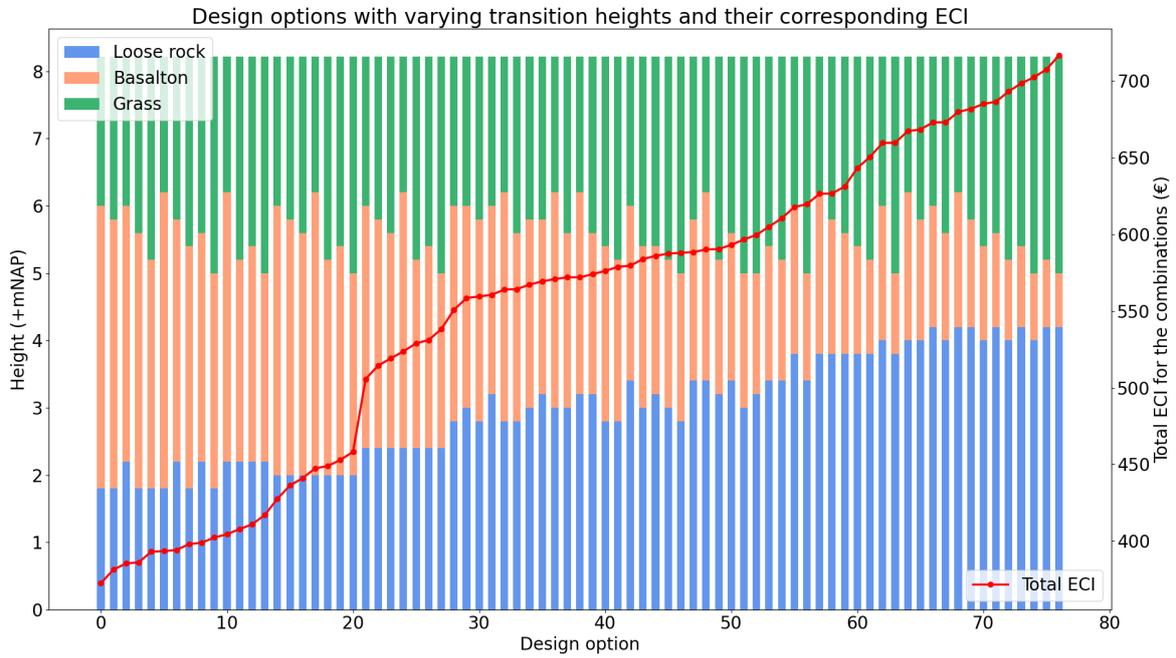
Figure 4.13: Design options with varying transition heights for loose rock, Basalton and grass revetment. Designs sorted by ECI, increasing to the right
