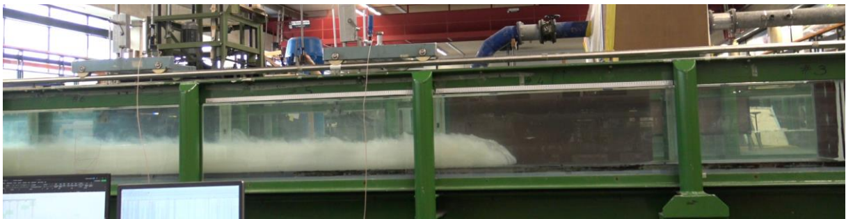
Figure 26 Picture showing the turbidity current developed behind the collector head (Test #5).
