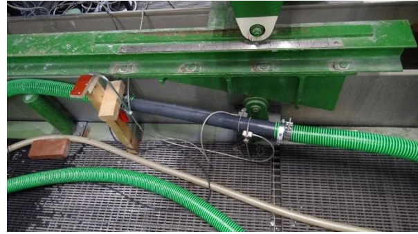
Figure 24 Attachment of the transducers to the PVC pipe.
