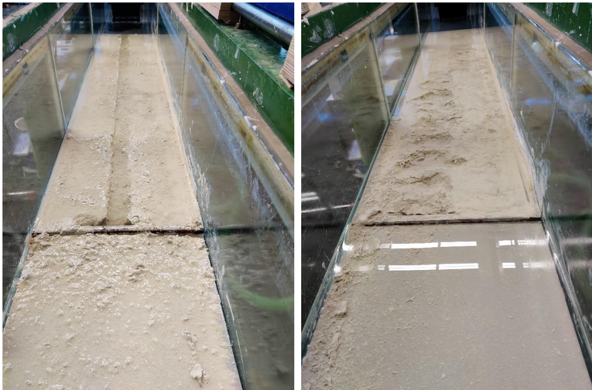
Figure 57 Erosion patterns of tests 8 (left) and test 13 (right).
