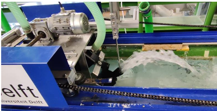
Figure 40 An experimental run in progress showing the water flowing out the collection duct while the EMS is measuring.
