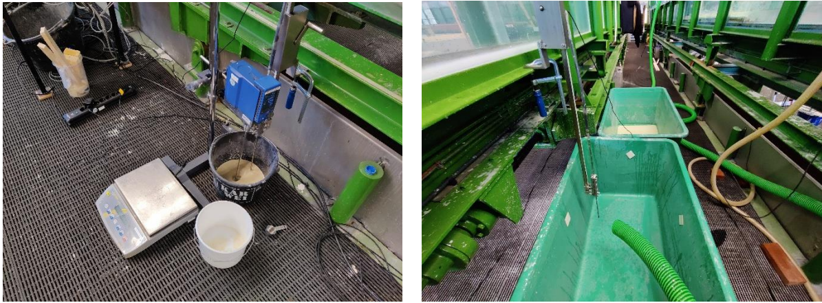
Figure 22 Calibration of the CCM (Left) and the position of the CCM during the experiments.
