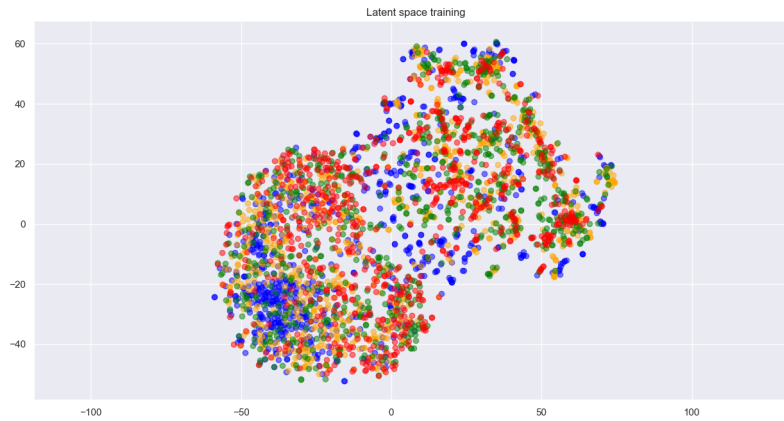
Figure 5.14: Latent space of training data with trajectories of different fishing gears. The blue, orange, green and red data points correspond respectively to mechanical dredges, beam trawlers 225 kW+, beam trawlers and other trawlers.
