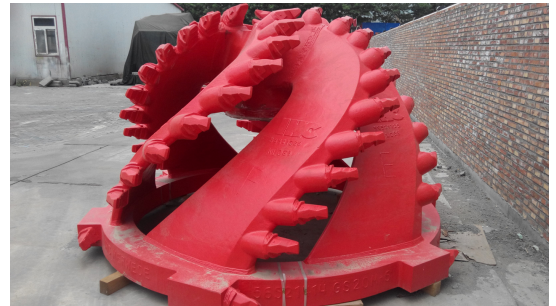
(b) Cutterhead for cutter suction dredges, IHC lightduty rock
