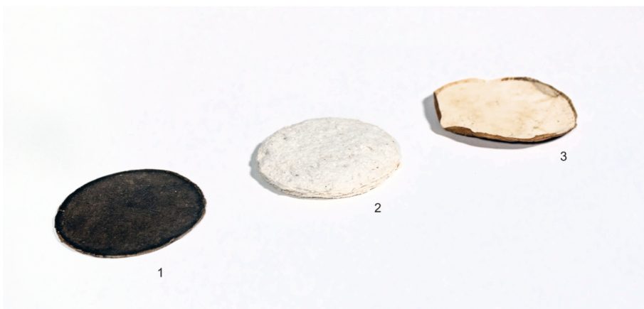
Figure 1. Three material samples. From left to right: 1.1 using fruiting bodies of white button mushrooms; 1.2 using fruiting bodies of bracket fungi; 1.3 from S. commune grown mycelium.
