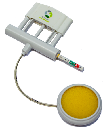
Figure 1.1: The Kiwi OmniCup The pump integrated in the handle allows for the creation of suction through a squeezing motion and simultaneously exertion of traction force.
