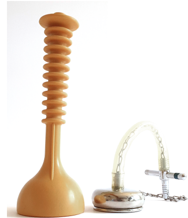
Figure 2.5: Side to side comparison of a pliable and rigid vacuum cup. Left: The Silc Cup, a pliable vacuum cup. Right: The original Malmström cup, a rigid vacuum cup.
