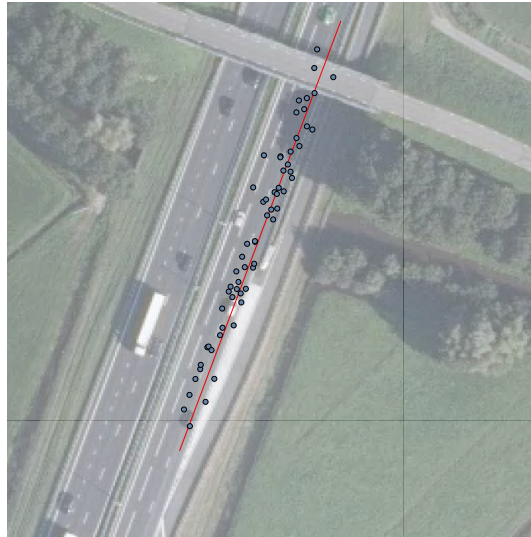
Figure 5.1: Using the centroids of events to check the precision of the smartphone GNSS by using the distance to the middle of the most right lane as a basis.
