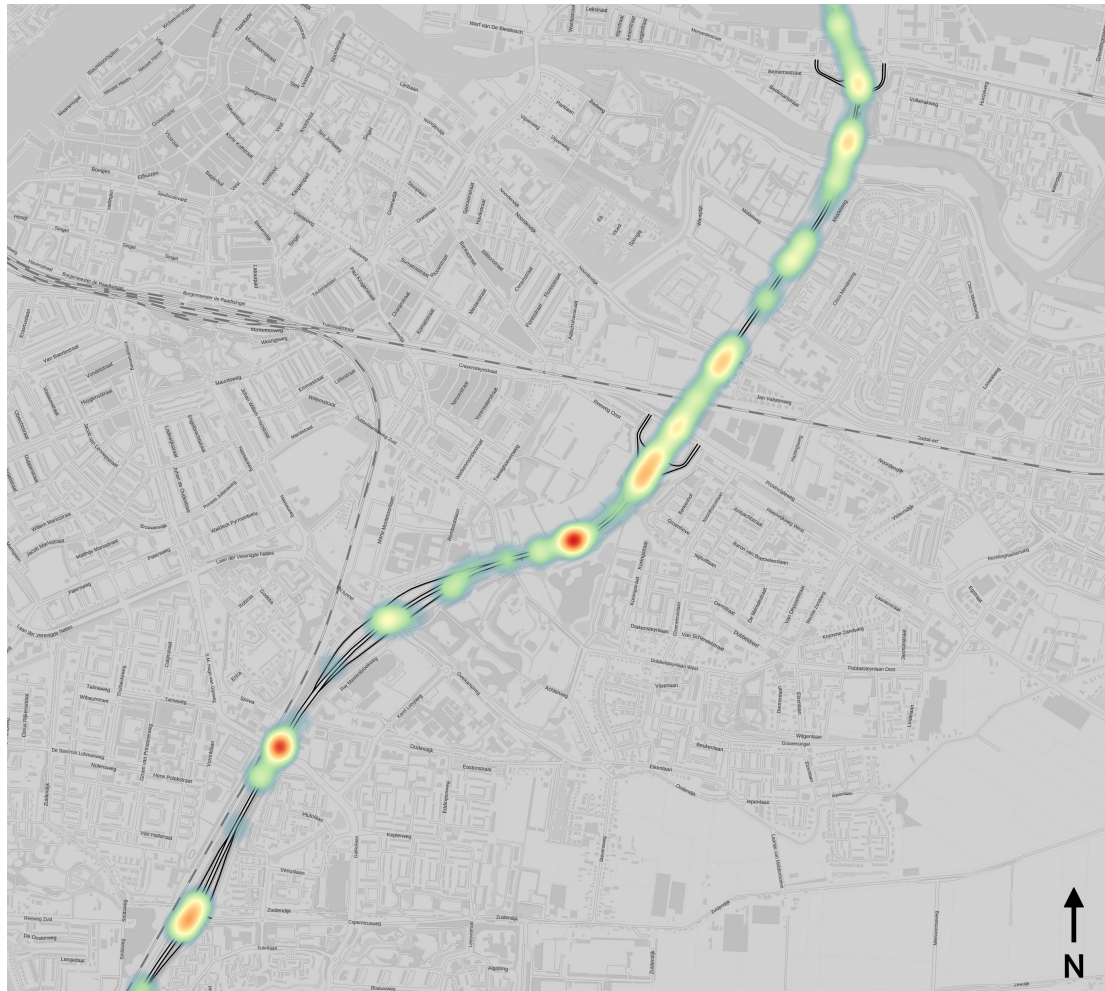
Figure 5.11: Visualizing the road pavement distresses and their severity.
