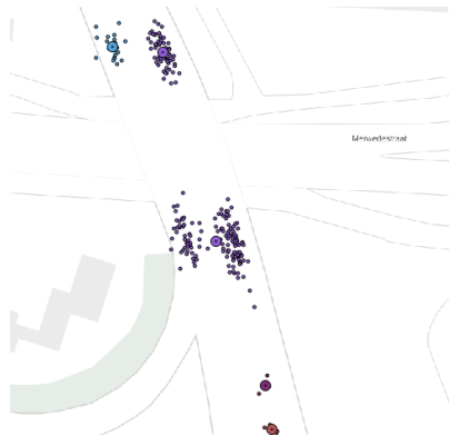
Figure 5.9: The creation of a cluster consisting of events from both road directions.
