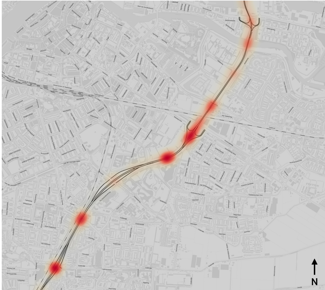
Figure 5.12: Visualizing the distribution of road pavement distresses in a heatmap.
