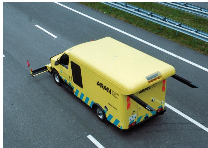
Figure 2.5: The ARAN of RWS in action. ( Rijkswaterstaat, 1996 )
