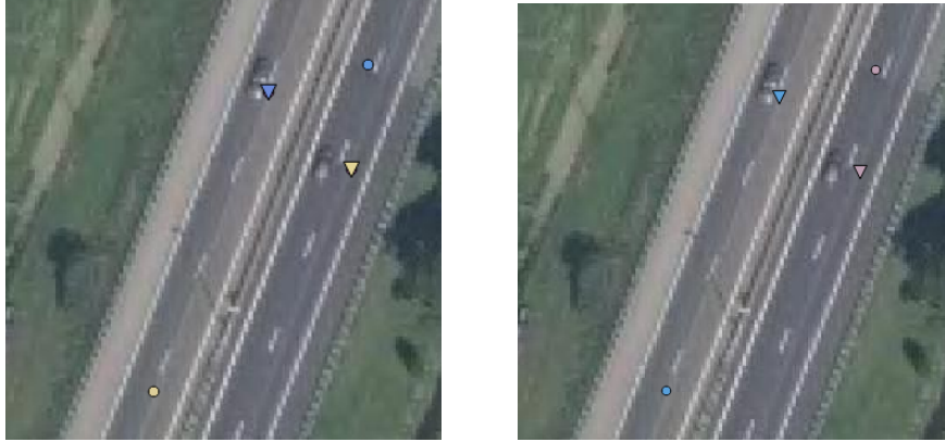
Figure 5.8: Connecting clusters shown as circles to the wrong hectometre post shown as triangles(left) and the result after fist connecting to the road centreline (right).
