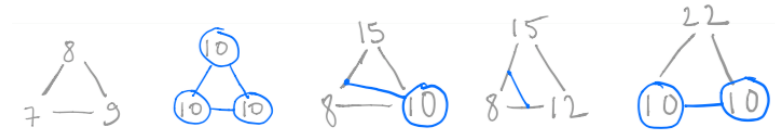
Figure 8.4: Different cases when extracting an isoline at elevation 10m for a TIN. The grey values are the elevation of the vertices forming one triangle, and the blue lines and vertices are the ones extracted for that triangle.
