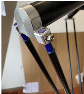
(b) The clamped TPU flexures on the Delta robot
