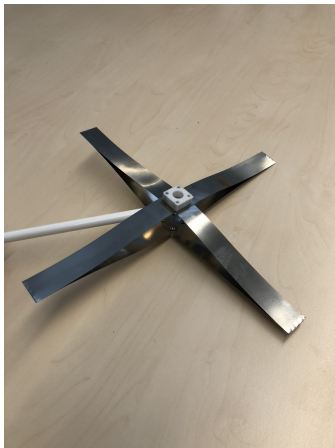
(a) A flat crossed leaf flexure. A pen is used to keep the two sides slightly spaced apart
