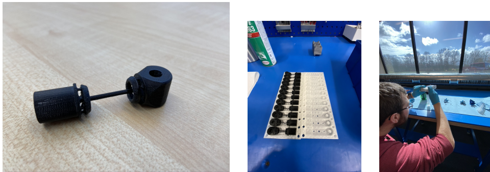
(a) The core of the flexure to pour around (b) A 3D printed mould with cores inserted. (c) Using a syringe to press the polyurethane into the mould.
