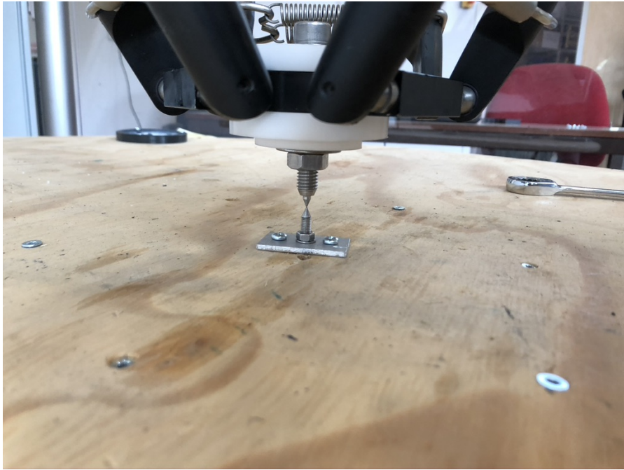
Figure C.5: The calibration of a point in 3D space to test the feed forward model of the delta robot with flexures.
