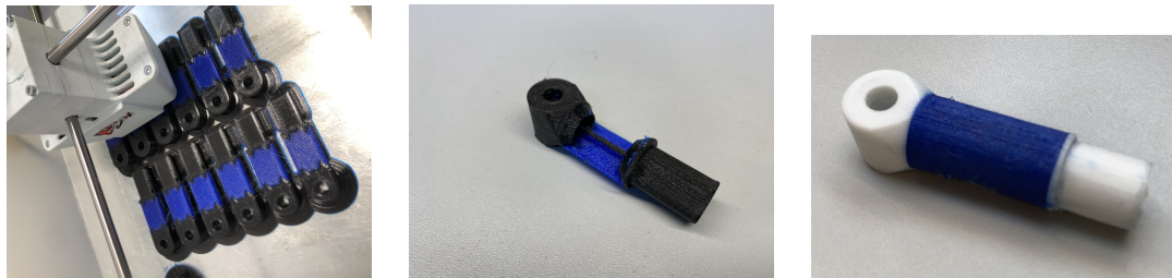
(a) A multimaterial 3D print of the flexures
