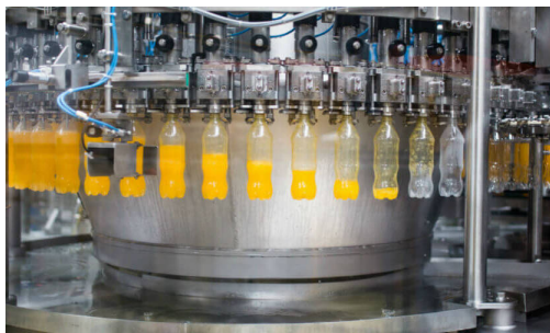
(a) Industrial bottle filling and handling machine [1]
