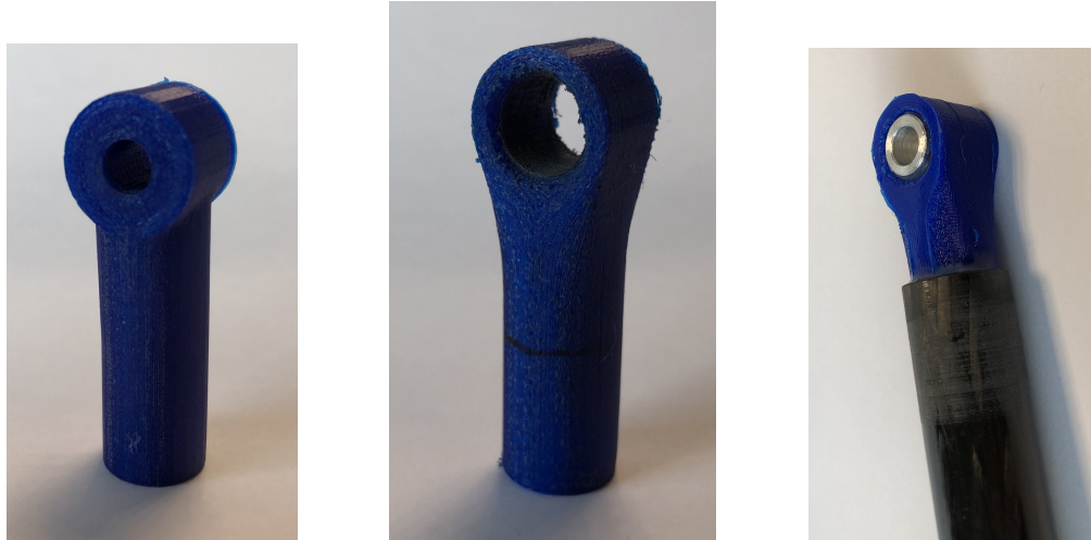
(a) The altered design, which can be printed flat on the table
