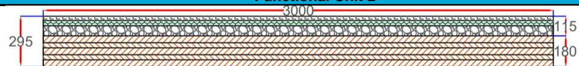
*j) CLT Solid Slab Element*
