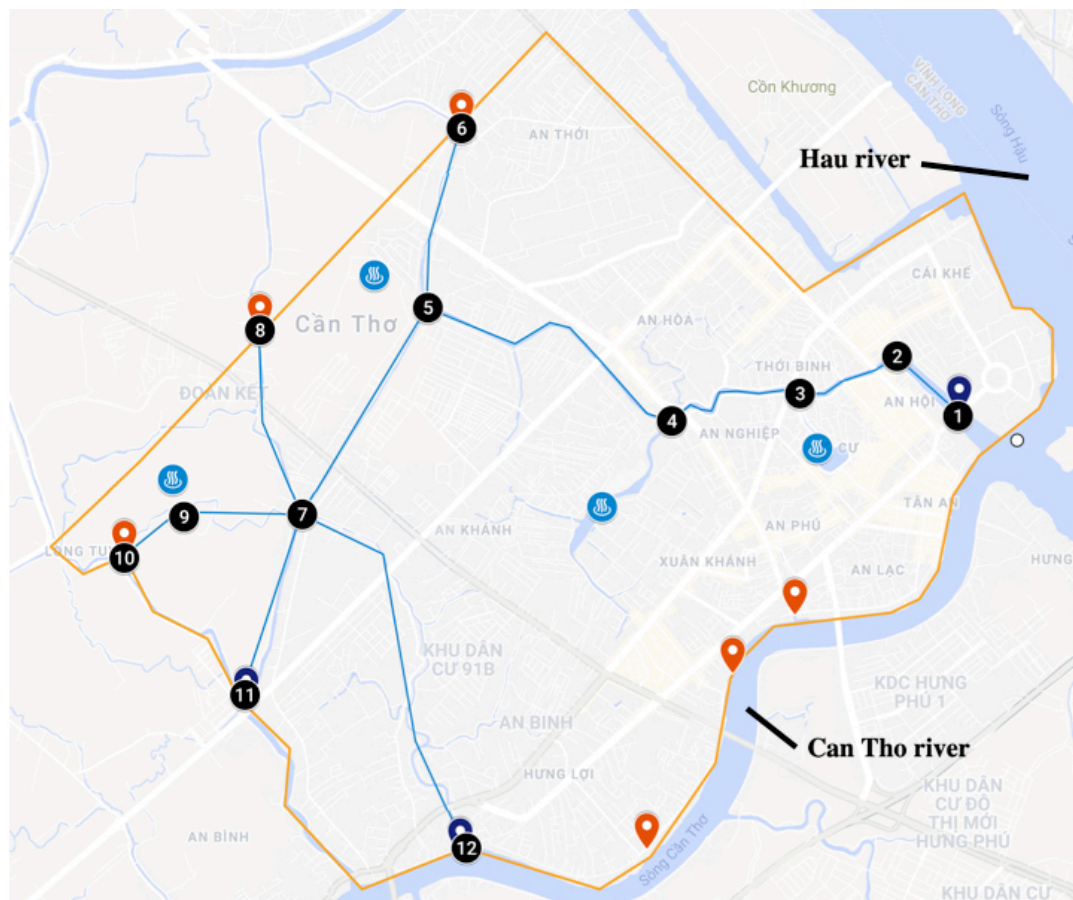
Figure 3.1: The polder area of Can Tho City is surrounded by the orange line. The blue lines indicate the modelled canals, with the nodes depicted as black circles. The red pin points at the border of the polder area are tidal gates only, while the blue pin points are tidal sluices including ship locks where ships can pass by. The retention lakes are shown as blue circles connected to node 3,4,5 and 9. Figure made using Google MyMaps.
