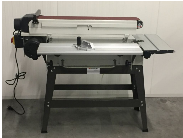
Figure 3.9: Actual Belt Sanding Machine (Heejan, 2021). Actual machine to be used in the test set-up. The sandpaper conveyor belt is the brown element that can be seen in the top of the figure, the motor of the conveyor belt consists of the black objects on the left, and the grey surrounding table can be used to place equipment on
