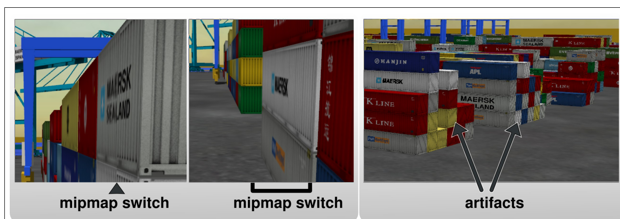
Figure 22: Artifacts with filtering techniques. The difference between bilinear and trilinear filtering (left) and the moire patterns when no filtering is done (right)
