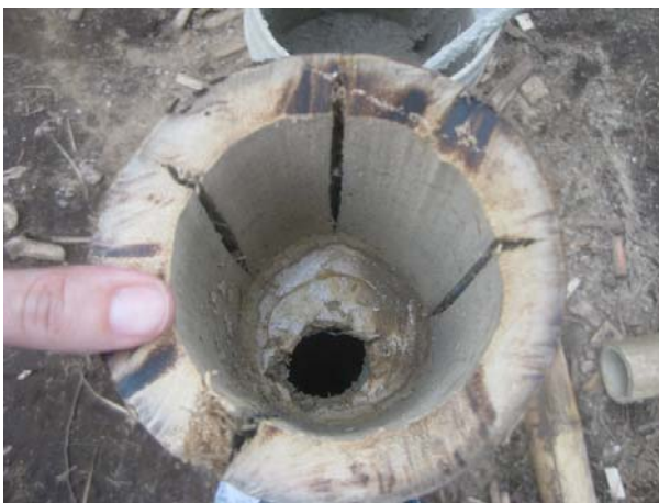
Fig 14. Culm wall thickness can vary widely in bamboo Guadua (CO2 Bamboo, 2010).
