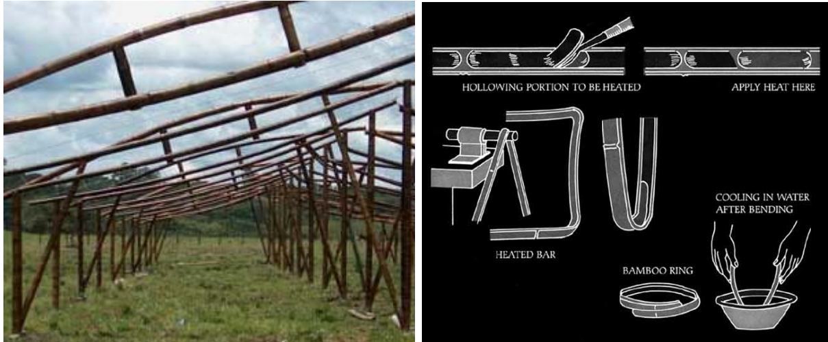
Fig. 36 Cold bent bamboo poles and warm bending process (Tonges, 2005).
