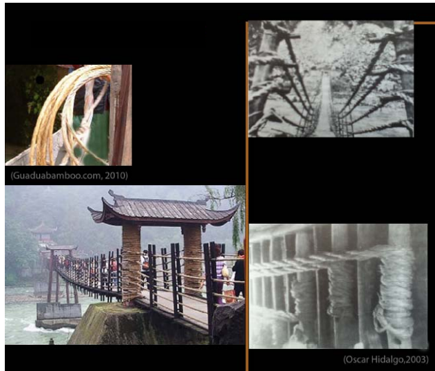
Fig. 52 Bamboo cable Diameter: 2-30cm Tensile strength: 1,863kg/cm 2 Carrying capacity (effective length 0.79m): 6 tons
