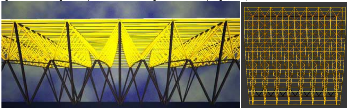
Fig. 39 Model of design for 27m span roof for playing field University of Pereira in Colombia (Tonges, 2005).
