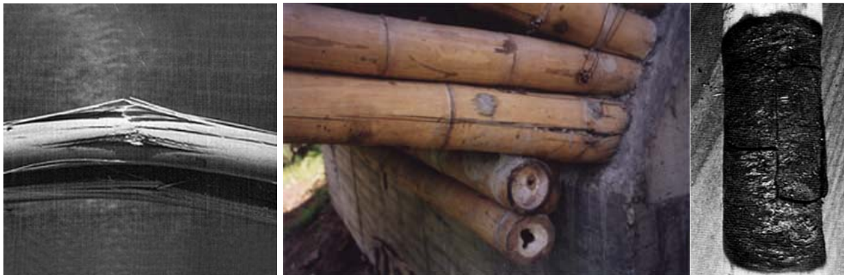
Fig.16 Fracture of pole (Tonges,2010) Fig. 17 Shear failure and combustion behavior (Ecobamboo, 2010).
