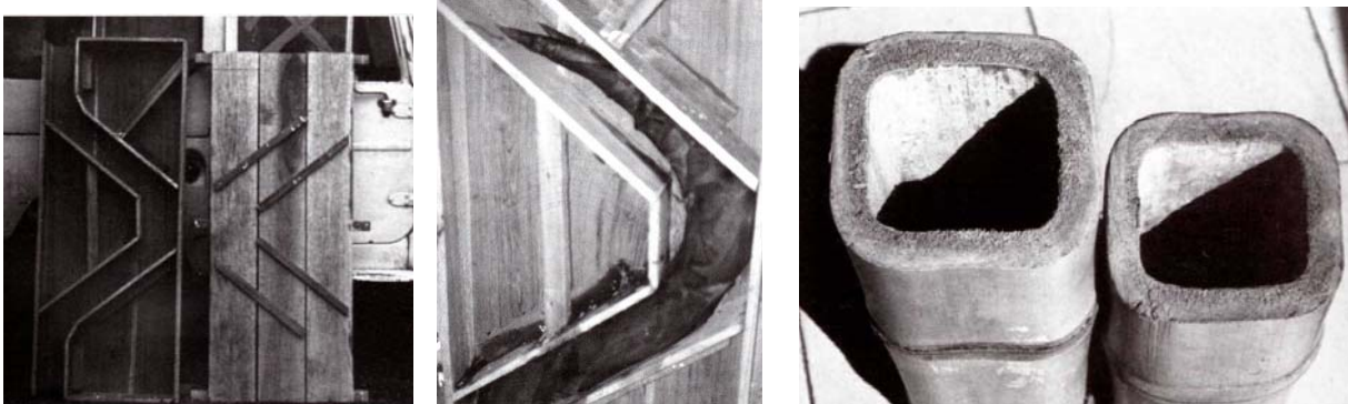
Fig. 35 Deformation trials- Wooden formwork and shoot growing, bamboo square cross-section (Hidalgo, 2003).
