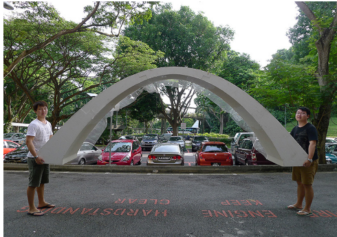
Figure 8 4 m span, 1:5 scale EPS composite arch prototype. The EPS foam has a Dryvit coating applied to the top and bottom sides. It is exceptionally light as a construction material and can easily be carried by two people. It is also structurally stable with a person standing on top.
