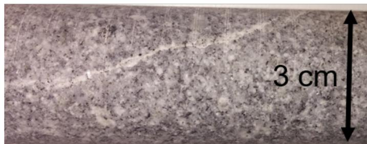
Figure 4.3: Fracture present in GRA\_2. A similar fracture was present in GRA\_3.
