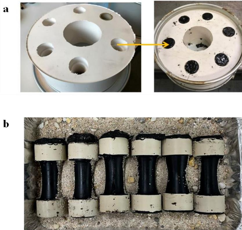
**Fig. 20 (a) The silicone mould with mortar and (b) mortar sample after demoulding**
