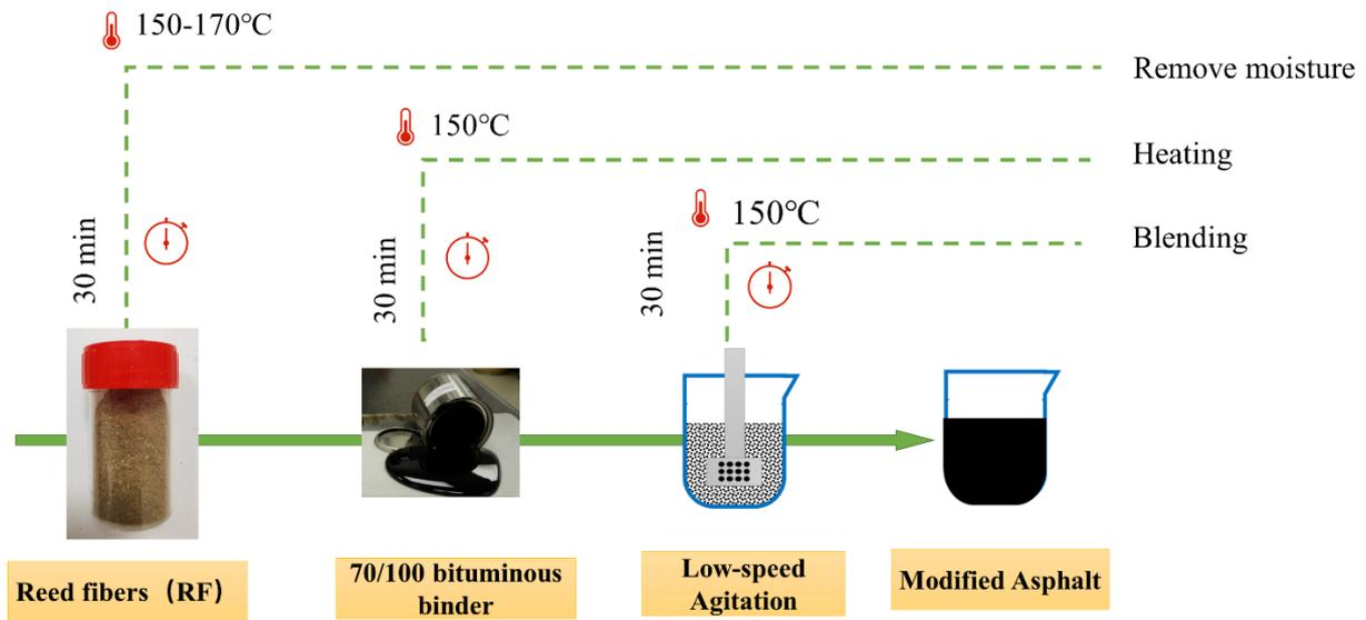
**Fig. 2. Preparation process of reed fiber-modified bituminous binder**
