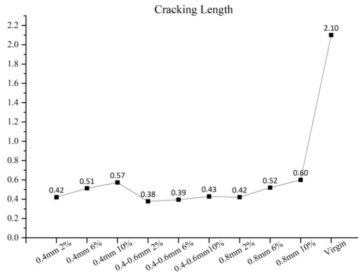
**Fig. 19 Crack length at failure**
