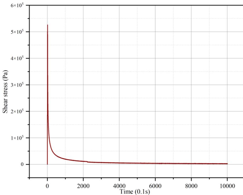
**Fig. 12. Relaxation test stress-time curve of 0.4mm 6% reed fiber**
