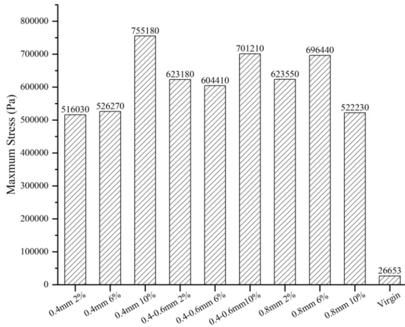
**Fig. 13. Maximum shear stress at relaxation test**
