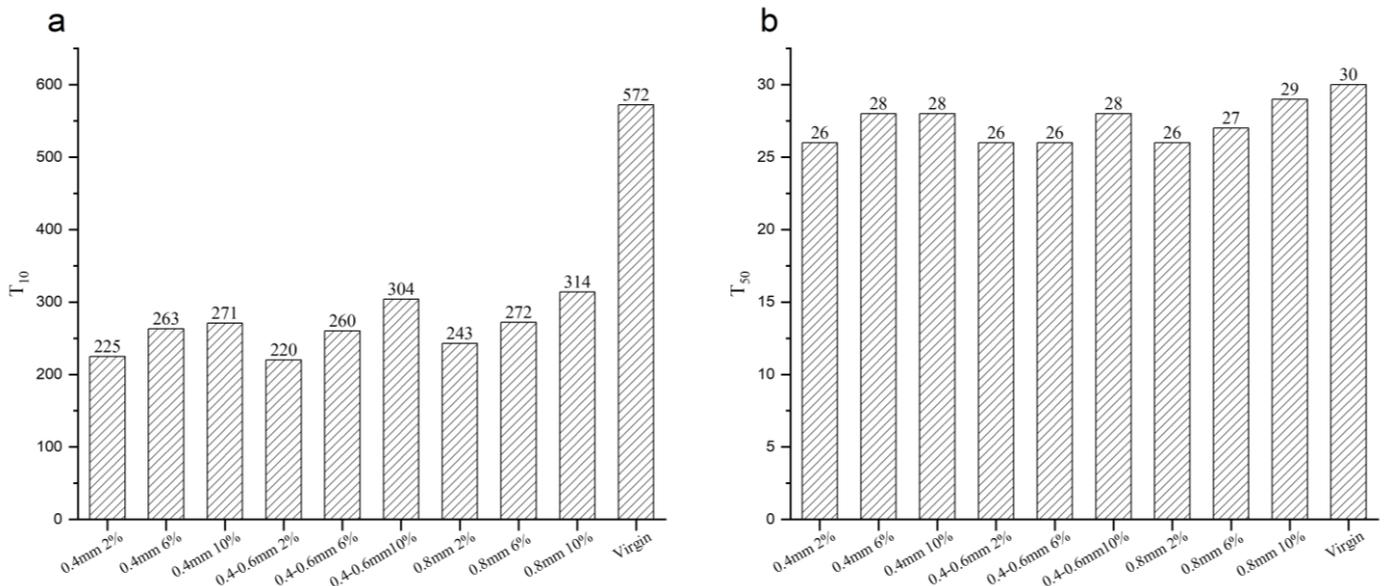
**Fig. 14. The time for the stress to return to (a) 10% and (b) 50%**
