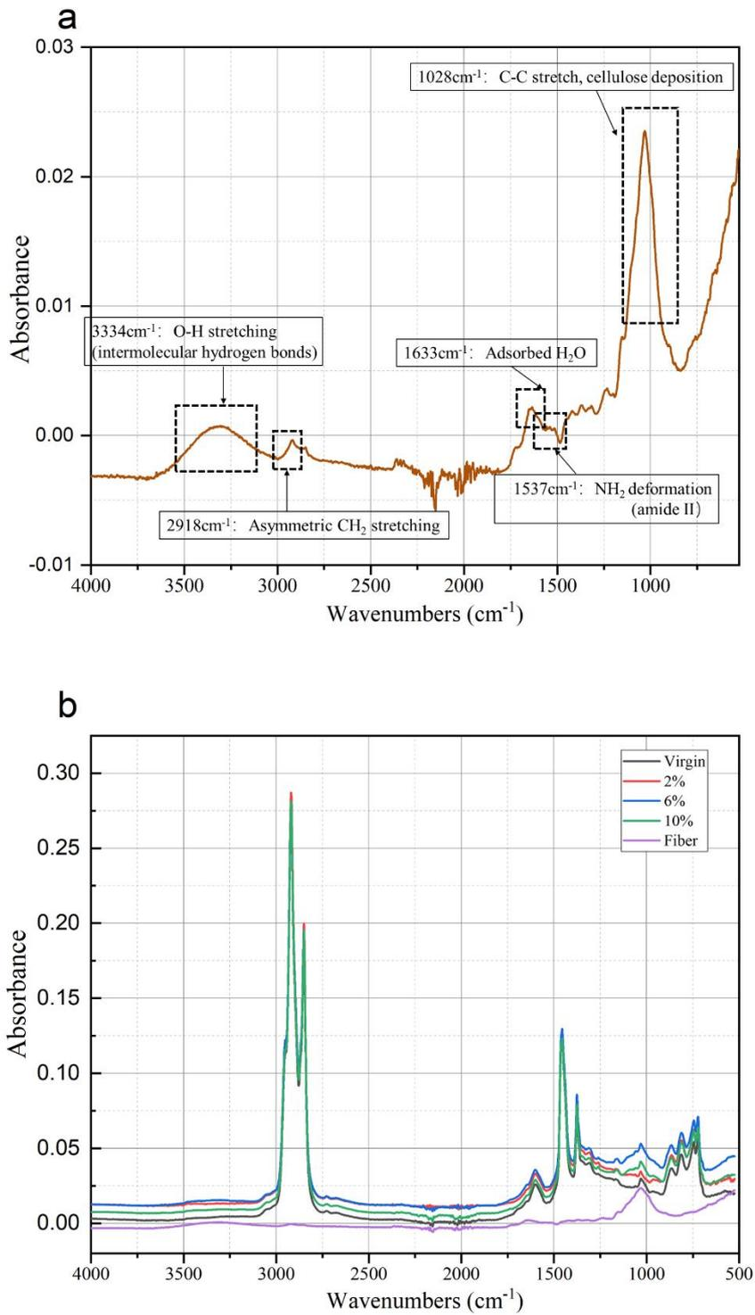
**Fig.4 The FTIR spectra of (a)pure reed fiber and (b)virgin bitumen, RFMB**
