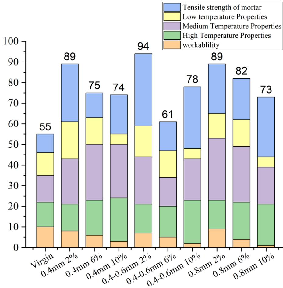
**Fig. 24 Rank value of different RFMB and virgin bitumen**
