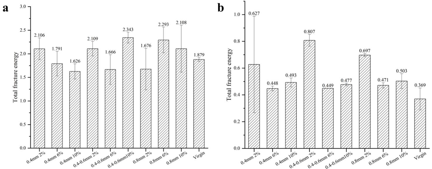
**Fig. 23. Fracture energy at (a)5°C ,(b)20°C**
