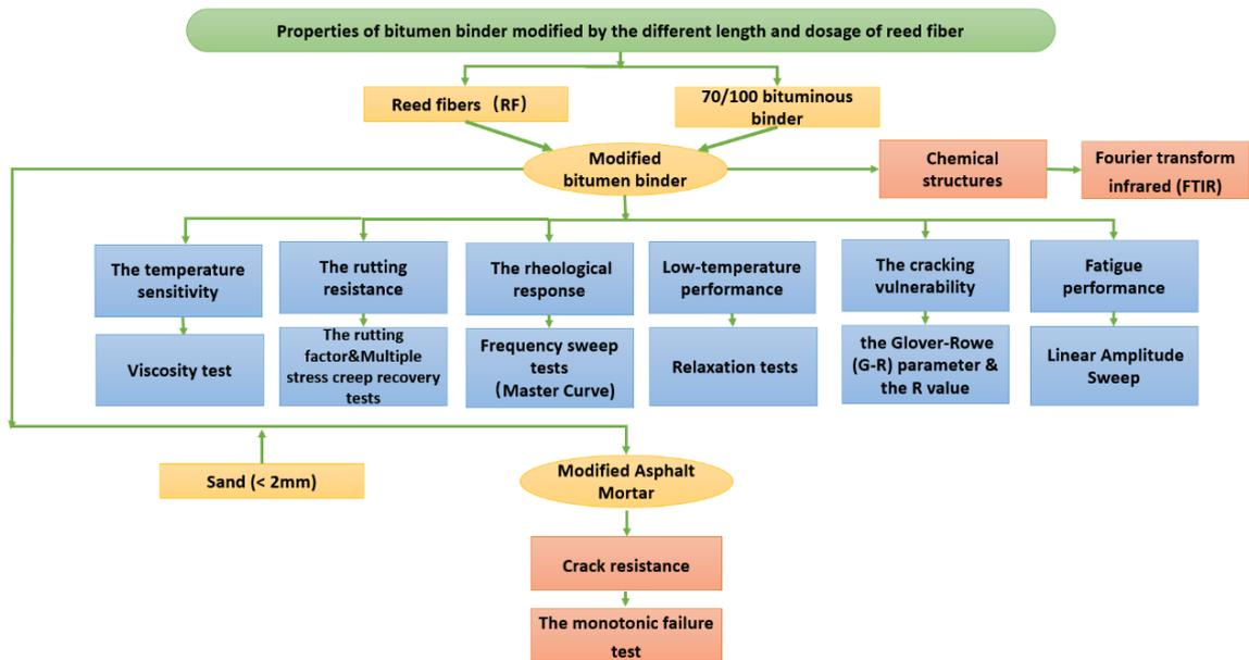
**Fig. 3. The framework of the experimental program**
