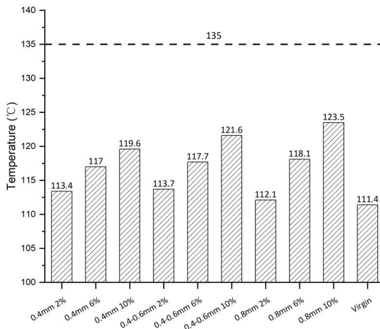
**Fig. 6. Temperature with a viscosity of 3 Pa·s per sample at 20 rpm**
