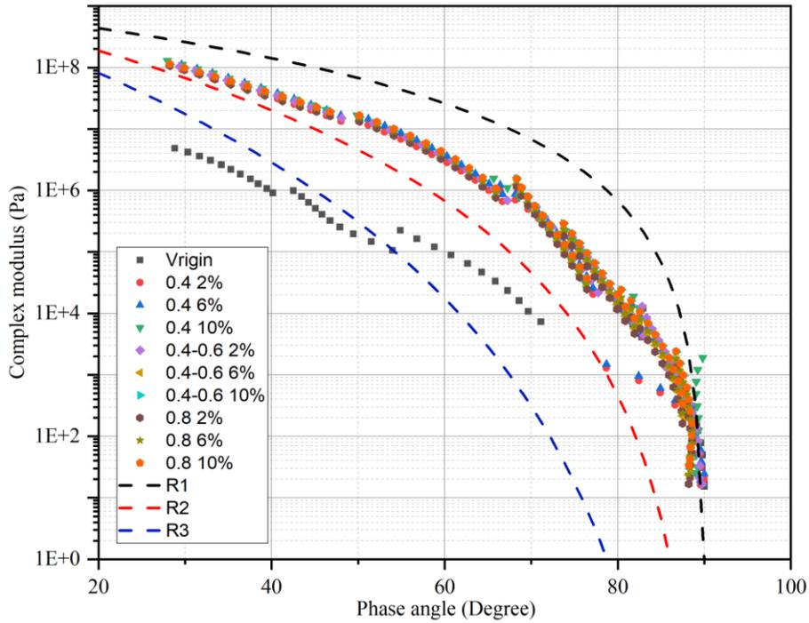
**Fig. 9. Black space diagram of rheological data for each sample**
