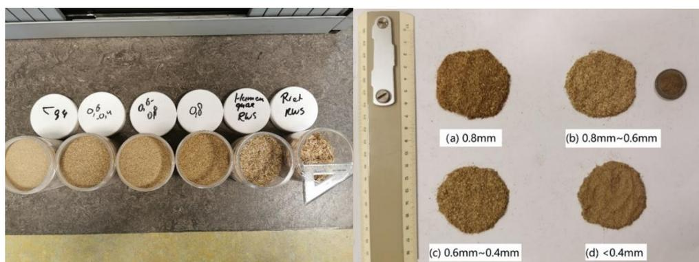
**Fig. 1. Reed fiber s' appearance (0.8 mm, 0.8 mm~0.6 mm, 0.6 mm~0.4 mm, and <0.4 mm).**
