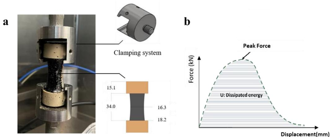
**Fig. 21 (a) Tensile test setup and (b) monotonic tensile Force-displacement curve**
