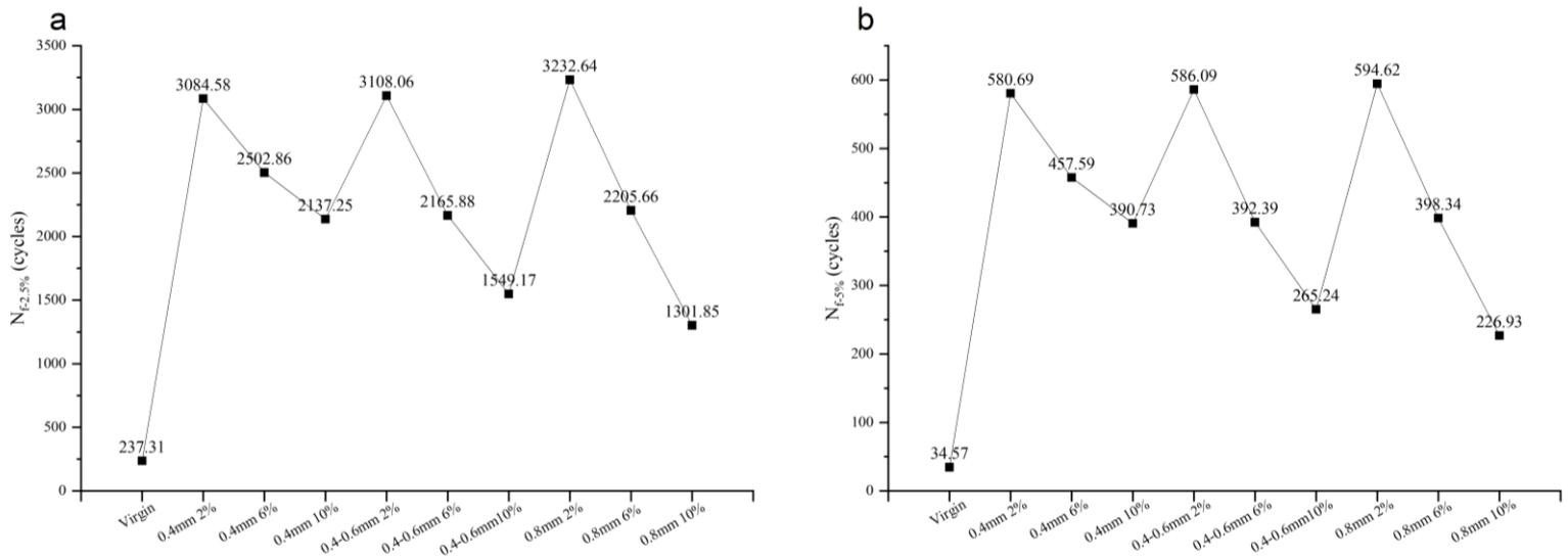
**Fig. 17 Predicted fatigue lives at (a) 2.5% and (b)5% strain amplitudes**
