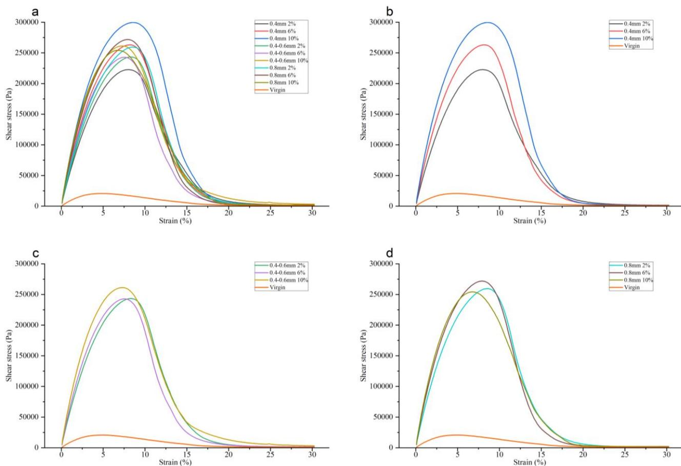
**Fig. 15. Stress-strain curves from the LAS test at different reed fiber length:(a) all (b)0.4mm; (c) 0.4-0.6mm; (d) 0.8mm.**
