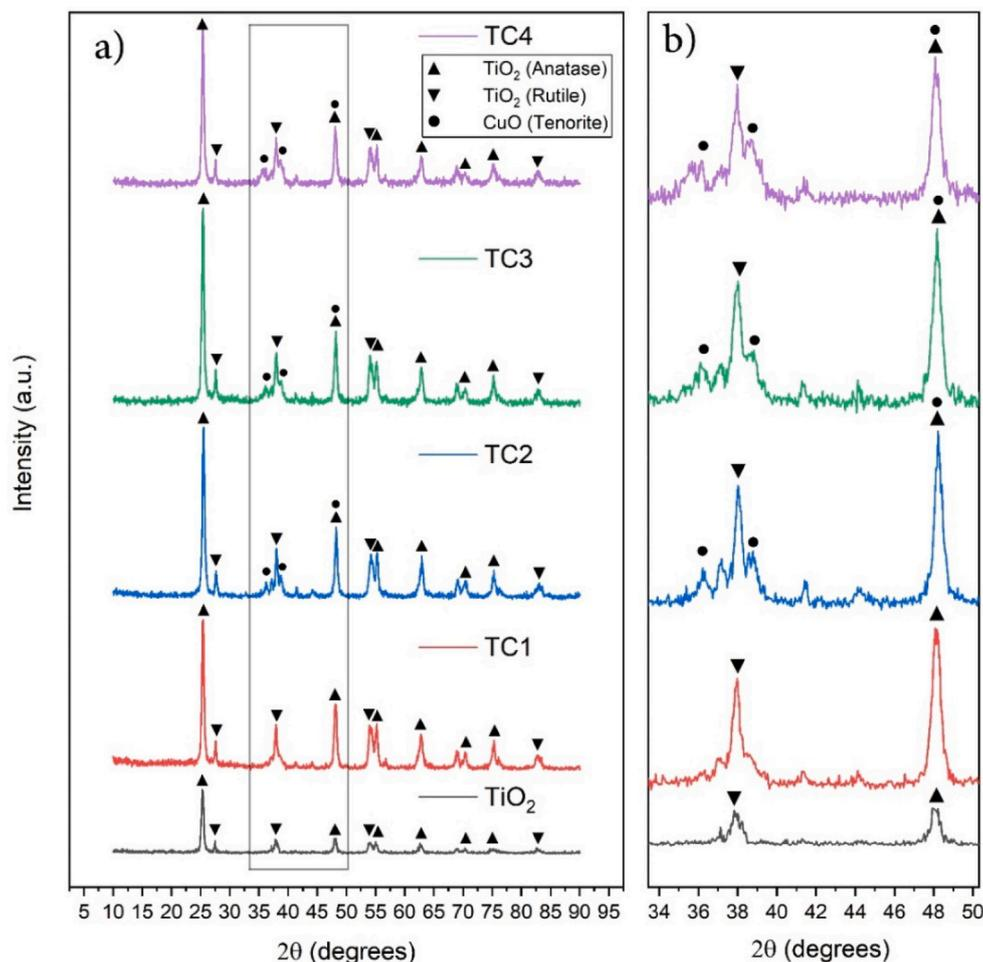
Fig. 4. XRD patterns of a) CuO-surface modified and bare TiO<sub>2</sub> photocatalyst samples and b) peaks correlated to CuO nanostructures.
