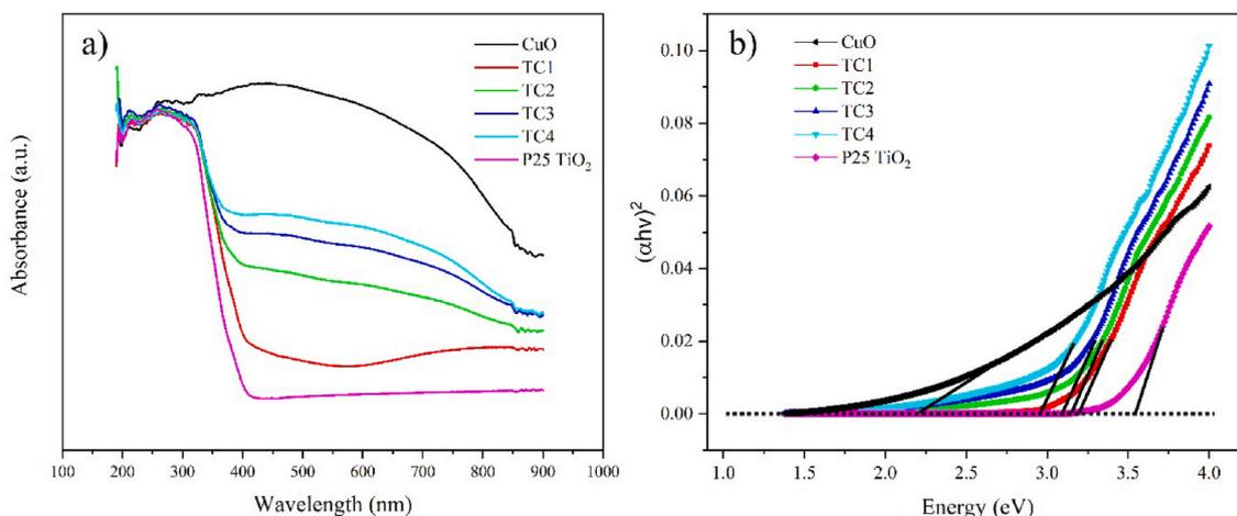
Fig. 7. a) UV-Vis diffuse reflection spectra, and b) Tauc plot of P25 TiO<sub>2</sub>, CuO nanoparticles, and CuO-surface modified TiO<sub>2</sub> nanoparticles.
