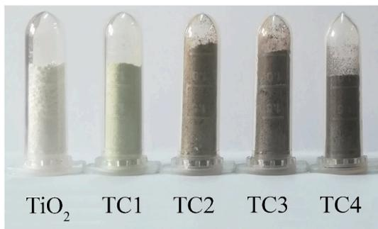
Fig. 2. Images of bare TiO<sub>2</sub> nanoparticles and CuO-modified TiO<sub>2</sub> photocatalyst samples.
