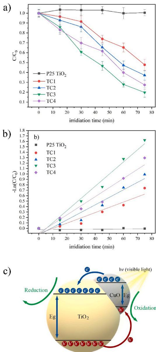
**Fig. 8.** a) Relative concentration changes of Amoxicillin under visible light on P25 TiO<sub>2</sub> and CuO-surface modified TiO<sub>2</sub> photocatalysts, b) First-order kinetic curves of visible light degradation of Amoxicillin under visible light on P25 TiO<sub>2</sub> and CuO surface modified TiO<sub>2</sub> photocatalysts, and c) schematic diagram of charge transfer on the CuO surface modified TiO<sub>2</sub> nanoparticles.
