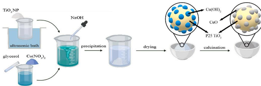
Fig. 1. Schematic diagram of the synthesis process of CuO surface modified TiO<sub>2</sub> nanoparticles.
