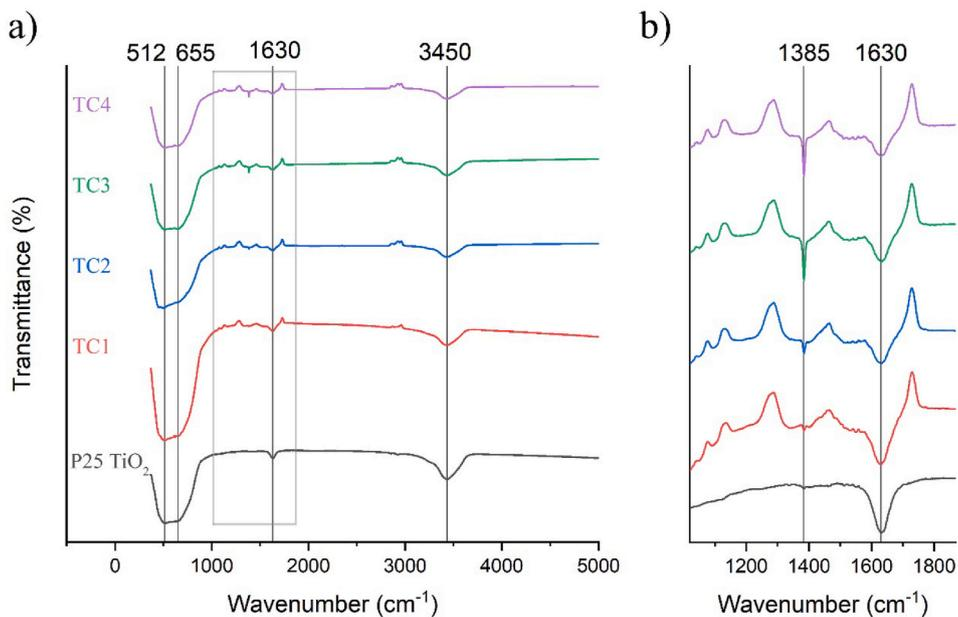
Fig. 6. FTIR spectra of a) CuO surface modified and bare TiO<sub>2</sub> photocatalyst samples and b) peaks correlating to CuO nanostructures.
