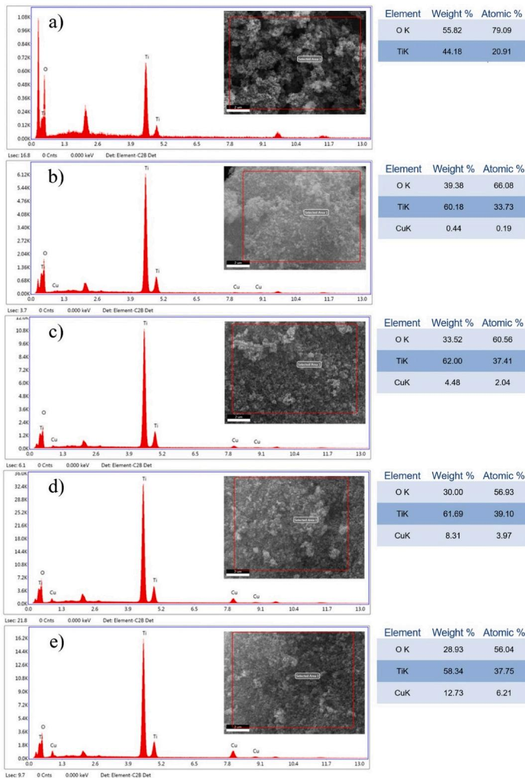
Fig. 3. SEM images and EDS chemical analysis of a) TiO<sub>2</sub>, b) TC1, c) TC2, d) TC3, and e) TC4 photocatalyst samples.
