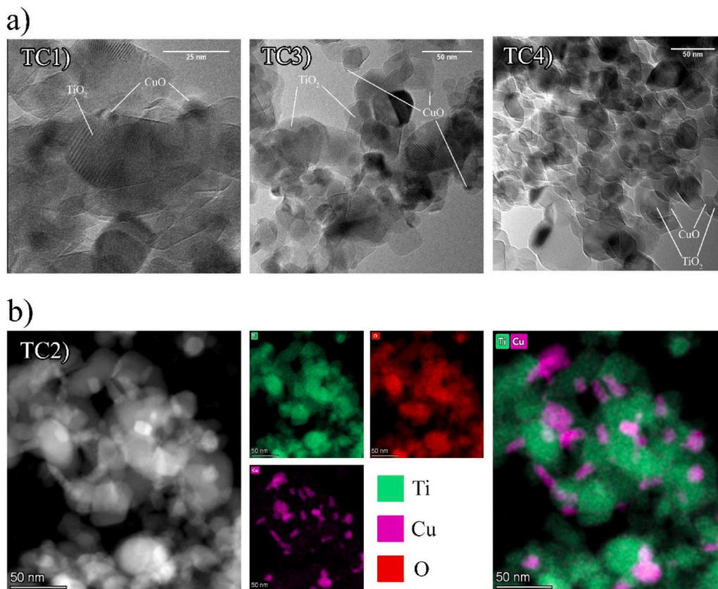
Fig. 5. TEM micrographs of a) TC1, TC3, and TC4 samples and b) HRTEM micrograph and elemental mappings of TC2 sample.
