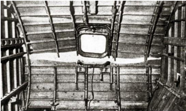
Figure 1.3: “The Comet” fuselage cracked during the tests. The crack started at a corner of a square window. The picture is taken from [16].
