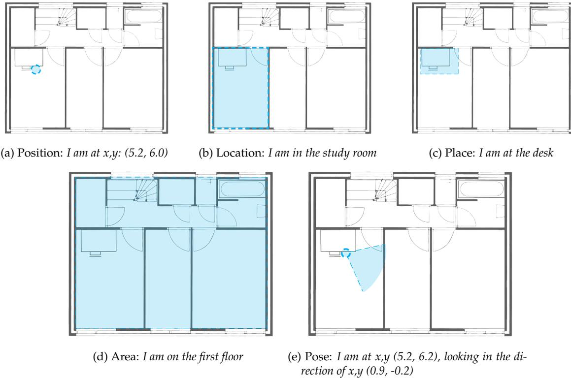
Figure 2.2: Differences between location; area; place; position; and pose.
