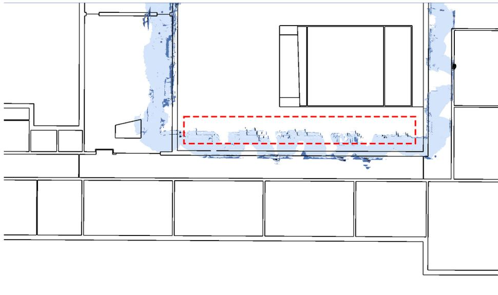
Figure 7.13: If one of the registrations gives an incorrect transformation, it is difficult to correct this with a 0.5 meter buffer. In this case, the y-value is off by approximately 5 meter. All walls (dark blue) inside the red rectangle will be removed because of the buffer.
