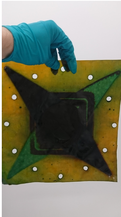
Figure D.2: A picture showing the fouling/damage of the membrane with the brown/black being iodine related fouling and the blue fouling being Prussian blue deposition.
