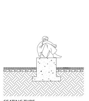
**SEATING TYPE:** - From 900 - 3000 mm thick color pigment mixed cast-in-place concrete.
