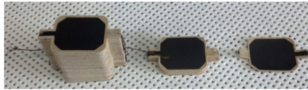
Figure 1.3. Stack unit DEAs form into a multistacked actuator [13].
