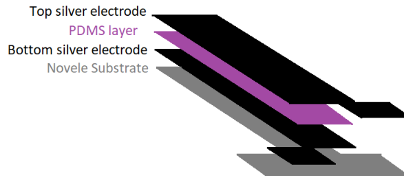
Figure 2.4. Structure of different layers in the single layer DEA.
