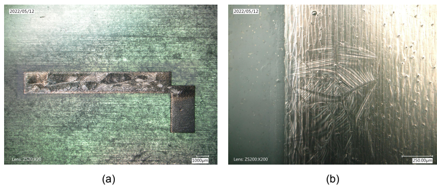
Figure 3.6. Observations under microscope for the wrinkled PDMS and close-up of wrinkles. (a) The inkjet printed PDMS layer full of wrinkles after 1min oxygen plasma treatment. (b) Close-up of the wrinkles on the PDMS.
