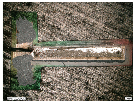
Figure 3.12. The single layer DEA (A2) having a top electrode with wrinkles but conductive.
