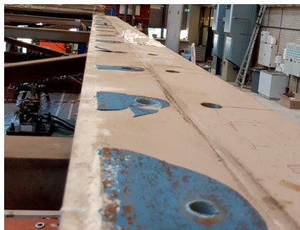
(a) Removal of the floor elements revealed substantial epoxy resin leakage at the steel-concrete interface.
