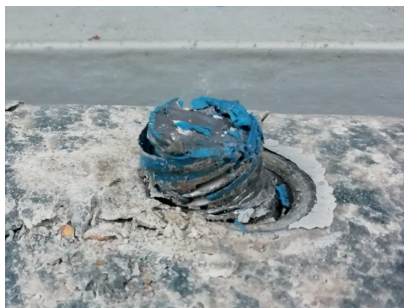
(a) Coupler with part of fractured bolt.
