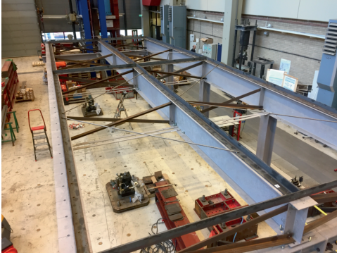
(a) Mock-up of steel beams, bracing system, and angle profile frames.
