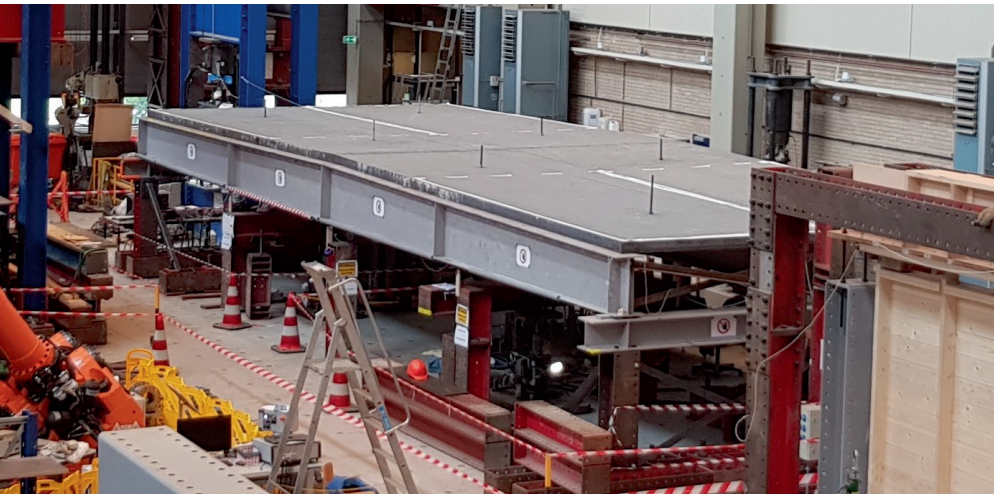
(e) Final assembly. The rods extending from the top surfaces of the floor elements were used for hoisting.
