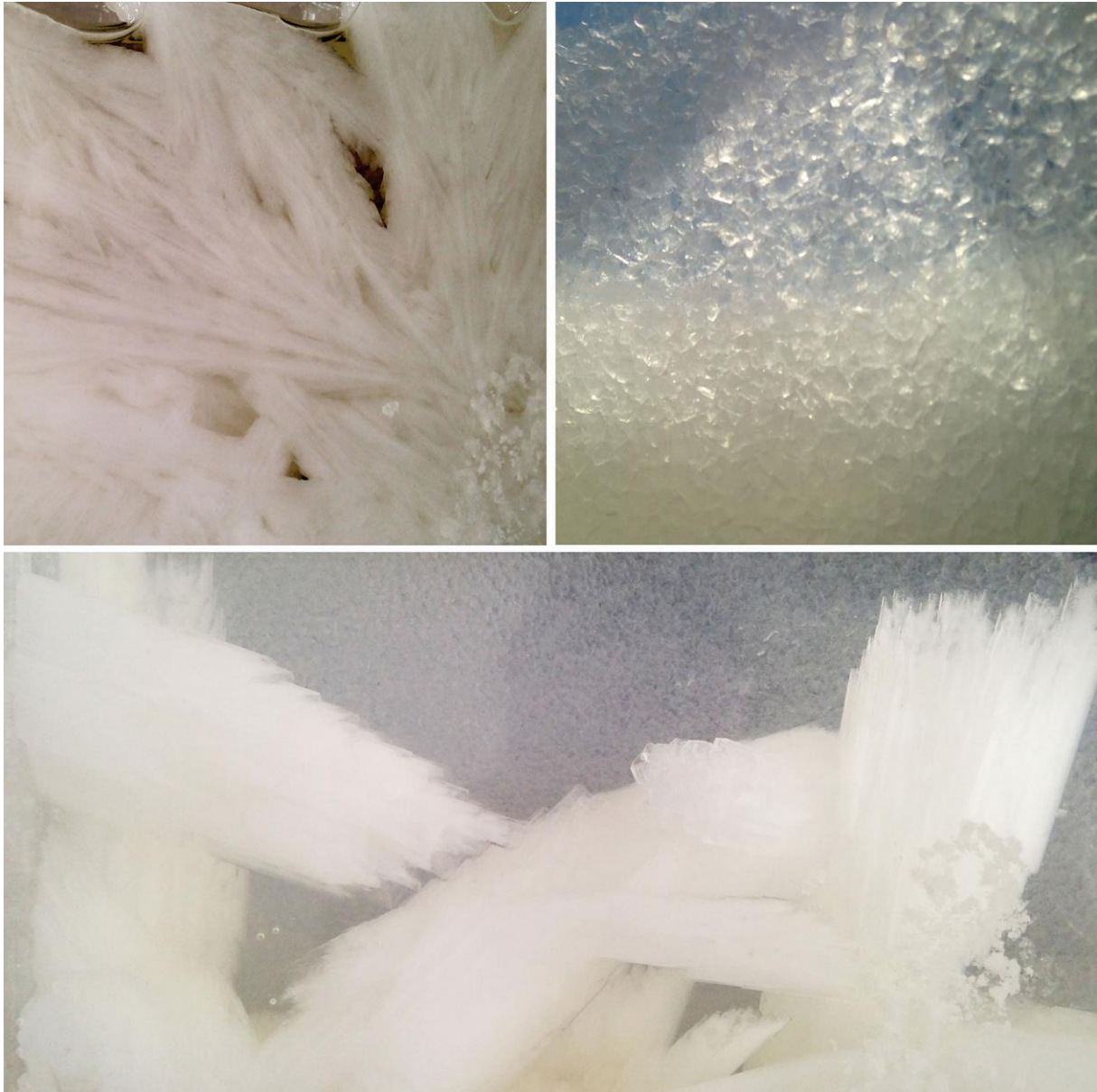
Figure 2: Top right: Beautiful crystals that start to emerge during the solidification process. Top left: Daylight passing through an insulating layer of Aerogel. Bottom: PCM's crystals in front of Aerogel.
