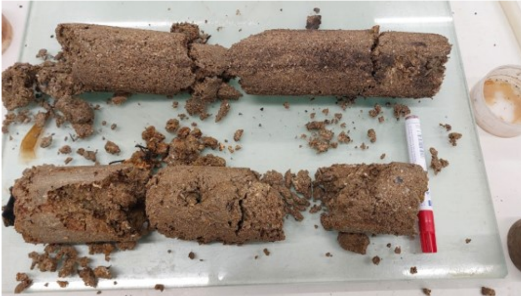
Figure E.3.2: Photos of the material from the sample tubes from which section were cut for shear box testing.
