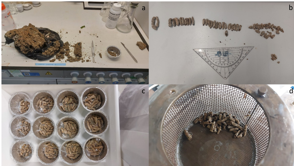
Figure E.1.5: Photos from the sample preparation and testing of single tubes using slake durability equipment. a) shows the procedure of dissecting the blocks into single tube parts. b) shows the sizing of the parts into their different classes. c) shows the three sample sets with each row a different sample set while the columns are the classes. d) shows the results after drying and testing.
