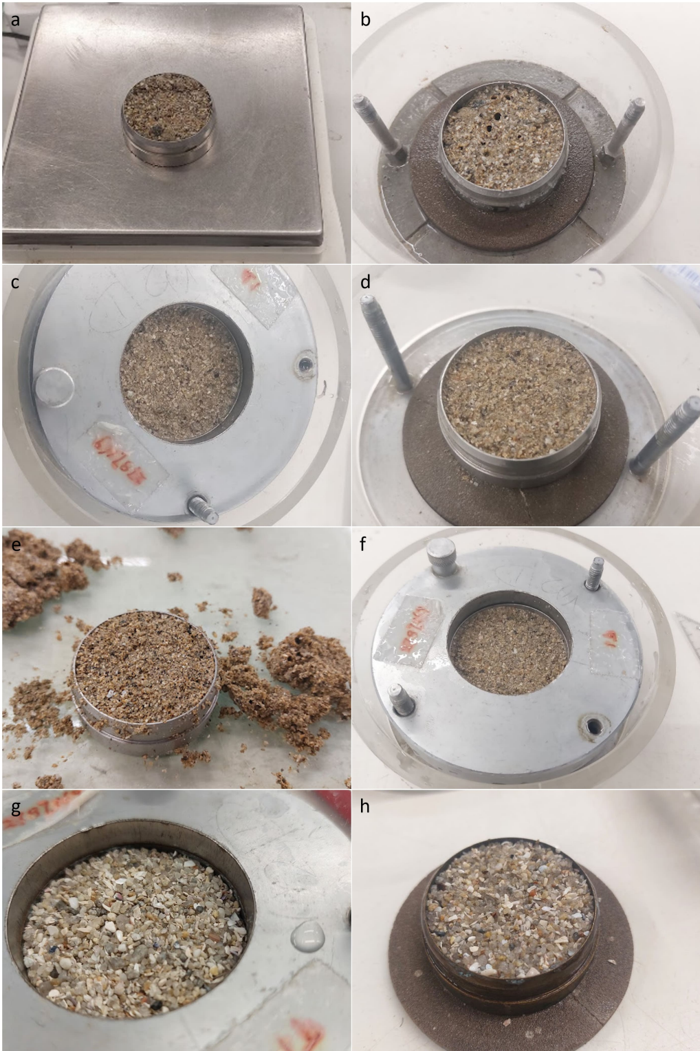
Figure E.2.2: Upper surfaces of the samples for oedometer testing before and after testing.
