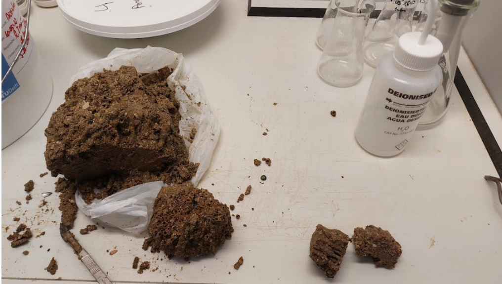
Figure E.1.1: Photo detailing the sample preparation for slake durability testing. Shown is a larger reef block from which smaller blocks are cut and the water bottle with which the blocks are rinsed.
