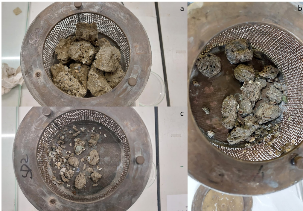
Figure E.1.4: Photos from the slake durability testing of sample 3 from location 5.2. a) shows the samples before testing, b) shows what is left of the sample after one cycle in the slake durability machine. c) shows the sample after two cycle of testing.
