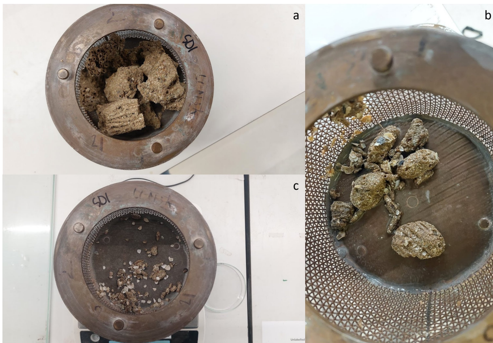
Figure E.1.3: Photos from the slake durability testing of sample 2 from location 4.1. a) shows the samples before testing, b) shows what is left of the sample after one cycle in the slake durability machine. c) shows the sample after two cycle of testing.
