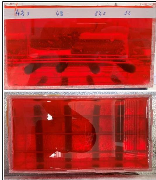
**Figure 1:** Placement 3 perpendicular rods above and beneath the targets to hold the targets in place. First: side view, Second: top view
