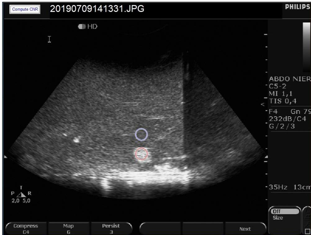
**Figure 3:** Captured ultrasound image with the red circle indicating the PVA target and the blue circle indicating the surrounding PVA phantom. The CNR in this case was 7.9991
