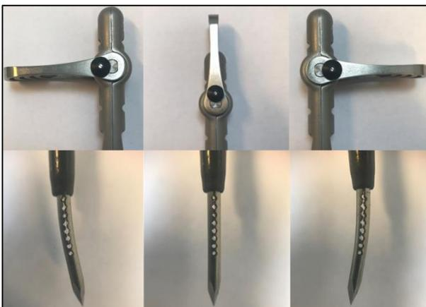
**Figure 3:** Steering mechanism of the steerable needle. Turning the lever clockwise results in a clockwise rotation of the needle tip and vice versa for turning the lever counter clockwise.
