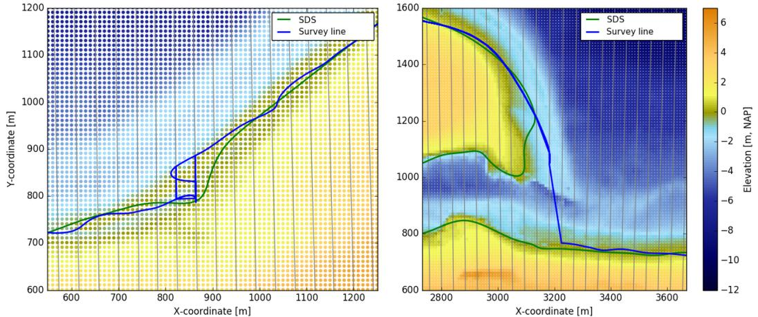
Figure 9: Zoom-in on the Landsat 5 benchmark case with the topography, the SDS (green) and the survey shoreline (blue). The left panel indicates the location near transect 21, the right panel indicates the location near transect 75. Please note that the scales of both panels are different.
