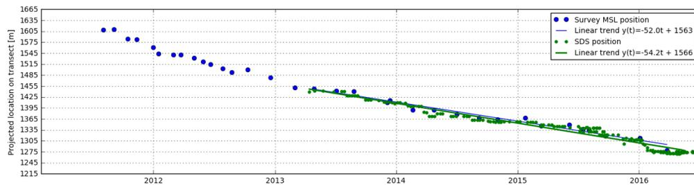
Figure 13: Timeseries of SDS positions the MSL contour lines obtained from the survey projected along transect 54. An OLS fit is made based on the information between 01-04-2013 and 01-07-2016.
