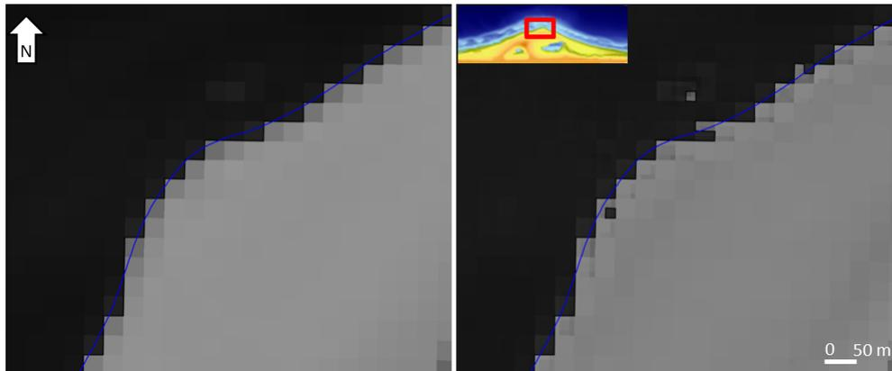
Figure 15: Effect of pansharping on the obtained SDS position. Top left shows the greyscale NDWI image and the obtained smoothed SDS position in blue on the Landsat 8 benchmark image. The right panel indicates the situation after pansharping.
