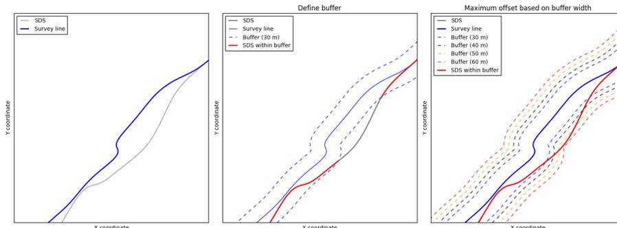
Figure 6: Buffer overlay offset routine to calculate the offset between the survey shoreline (blue) and the SDS (grey) using a buffer polygon (dashed line). The offset between the survey shoreline and the SDS is defined as the buffer that encloses 95% of the SDS.
