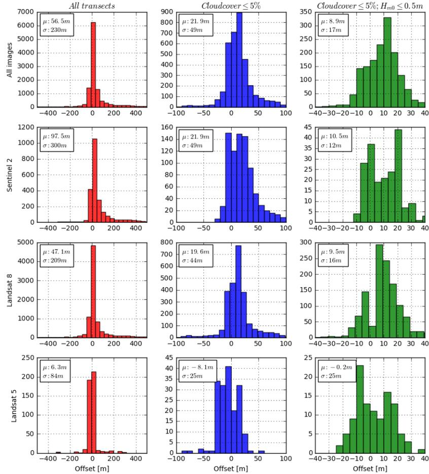
Figure 10: Overview of the offset calculation between all SDS positions and their concurrent survey shorelines. The first row contains the offset values for all satellite missions, the other rows contain the offset values per satellite mission. The second column indicates the result after filtering transects on local cloud cover, the third column indicates filtering on cloud cover and nearshore wave height. Please note the different x-axis limits per filter, which are the same for all missions.
