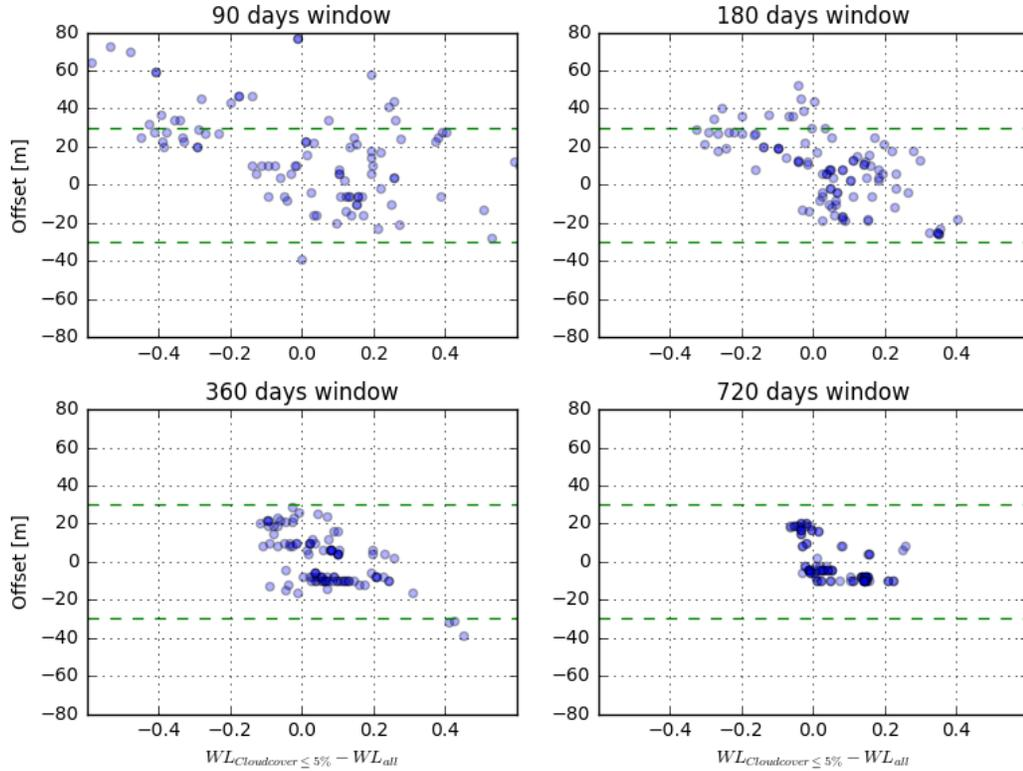
Figure 16: Effect of the image composite moving average time windows on the difference between the water level observed on the underlying cloud free images ( $WL_{Cloudcover \leq 5\%}$ ) and on all underlying images ( $WL_{all}$ ) within a time window in relation to the offset value. All values are based on the values found at the first transect. The Landsat pixel resolution is indicated in green.
