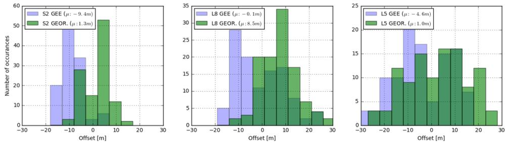
Figure 11: Overview of the offset calculation related to georeferencing before (GEE) and after georeferencing (GEOR.) for Sentinel 2 (first panel), Landsat 8 (second panel) and Landsat 5 (third panel).
