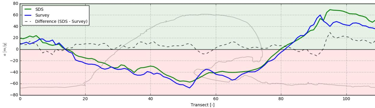
Figure 14: Alongshore rate of shoreline change ( $a$ ) based on the SDS position (green) and the survey MSL contour (blue). The black line indicates the difference between  $a_{SDS}$  and  $a_{Survey}$ . The MSL contour line from the survey conducted on 03-08-2011 is plotted in grey as a reference.
