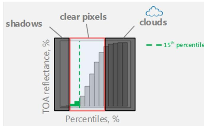
Figure 7: Principle of the image composite technique based on the distribution of all TOA reflectance values within the image composite time window per pixel. The 15<sup>th</sup> percentile value is used throughout this study to obtain a composite image. Adjusted from: Donchyts et al. (2016)
