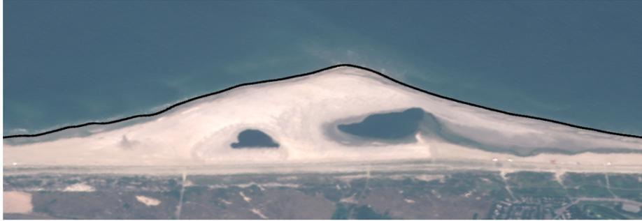
Figure 4: Satellite image acquired by the Sentinel 2 satellite acquired on 12-03-2015 10:33:27 (GMT) for the Sand Motor study site. The derived SDS is plotted in black.
