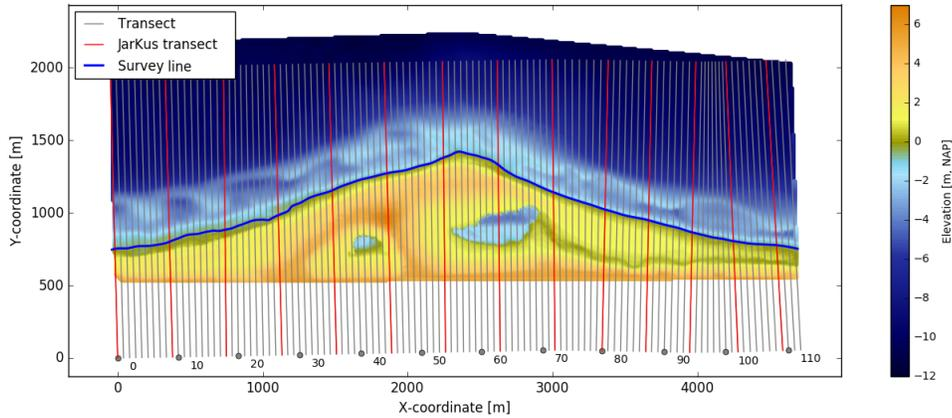
Figure 5: Interpolated topographic elevations and reconstructed survey shoreline for the 16-07-2015 Sentinel 2 satellite image. The measurement campaign to obtain the topography was conducted between 15-07-2016 and 17-07-2016. The transect system is indicated in grey and the JarKus transects are indicated in red. Every 10<sup>th</sup> transect origin is indicated with a grey dot. Elevations are with respect to NAP, the national datum, which is about MSL.
