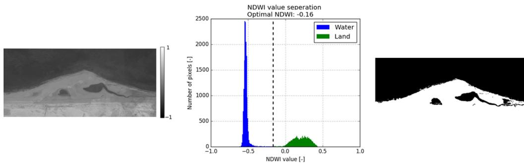
Figure 3: NDWI greyscale image (left), NDWI histogram (middle) and resulting binary image (right) for a Sentinel 2 image acquired on 12-03-2015 10:33:27 (GMT). An optimal threshold value of -0.16 classifies the NDWI values into water (blue) and land (green) pixels.
