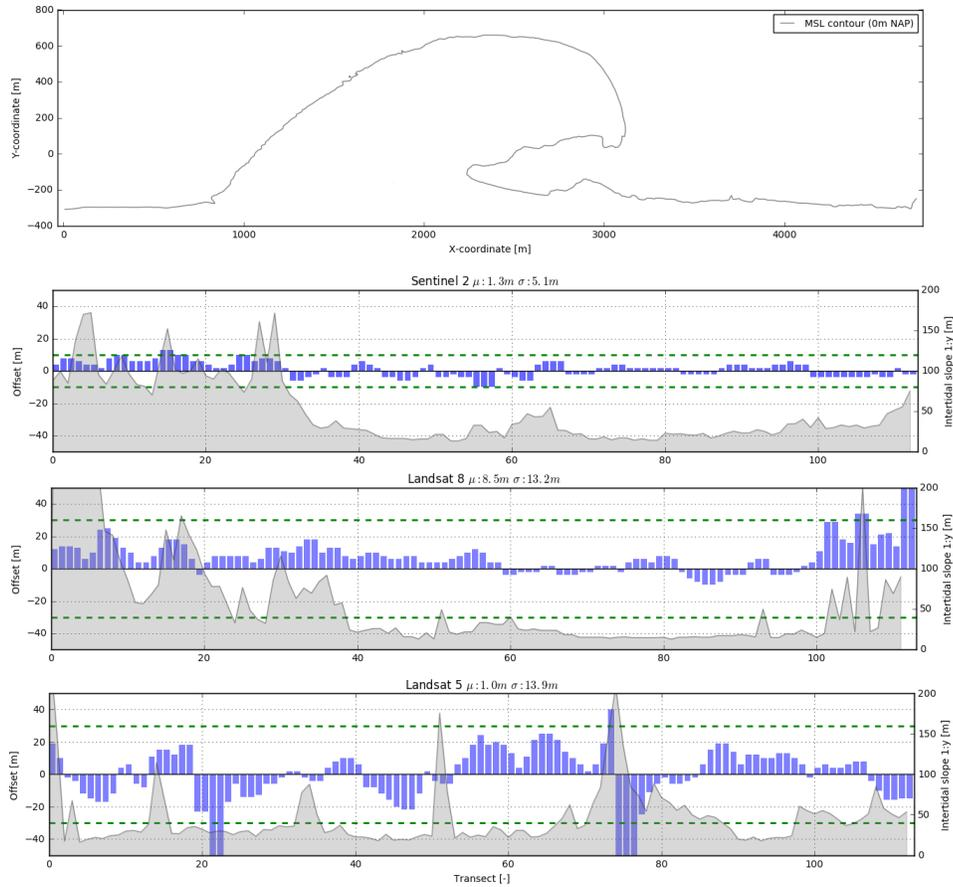
Figure 8: The top panel indicates the MSL elevation contour of the survey conducted on 03-08-2011. Offset result per transect for the Sentinel 2 (second panel), Landsat 8 (third panel) and Landsat 5 (bottom panel) benchmark cases. The image pixel resolution is indicated in green, the inter tidal beach slope per transect is plotted in grey.
