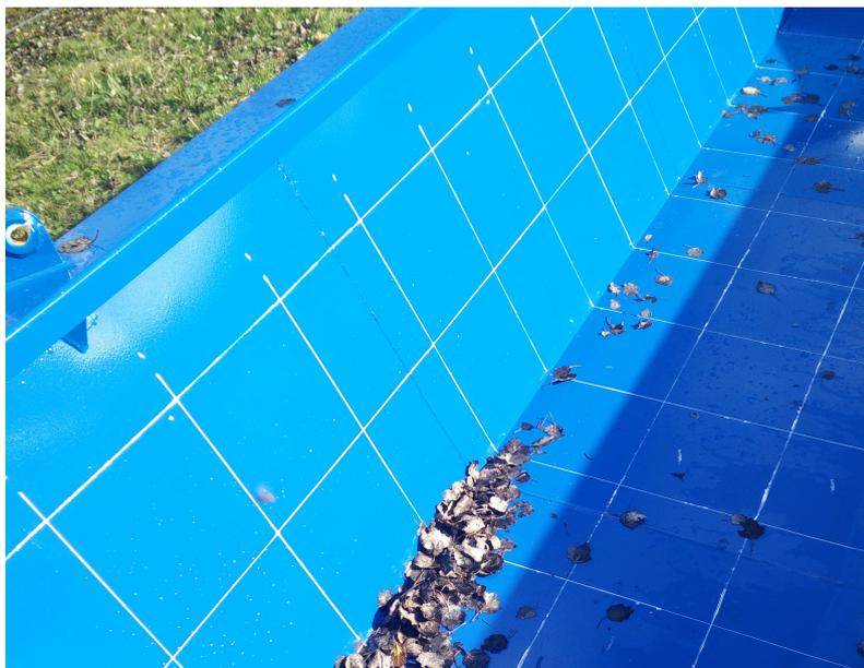
Figure 7.2: A grid, painted on the inside of the mock-up, that is used to do accurate on-board measurements.
