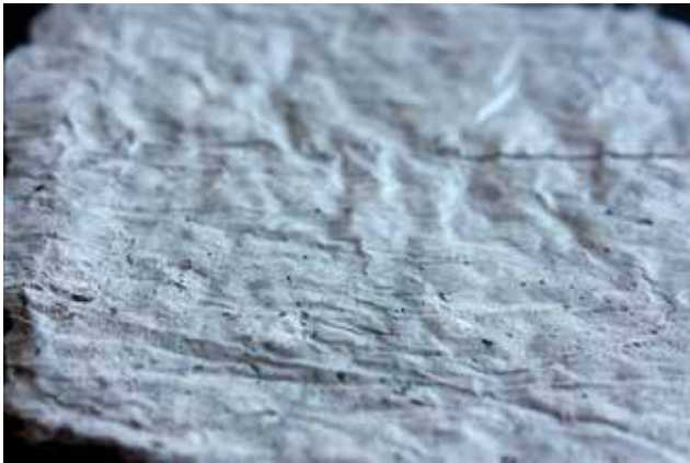
Figure 6. Sample of cellulose fibers mixed with flexible acrylic
