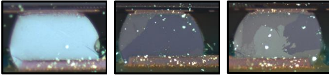
Figure 5: Single and Oligocrystalline Solder Joint
