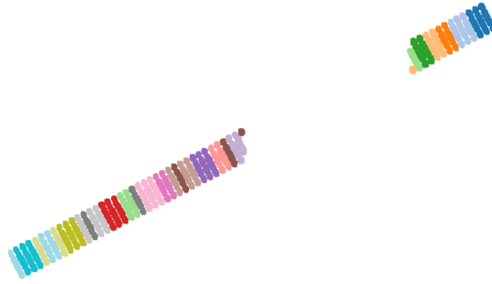
Figure 3.12: Clustered point cloud showing individual sleepers (colours are random, each sleeper is one cluster).
