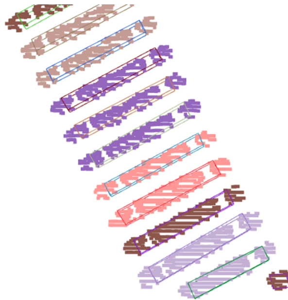
Figure 3.13: Filter bounding boxes superimposed on clustered sleepers. Random colours, each sleeper is one cluster.
