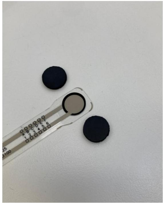
Figure 57. FlexiForce A201 sensor and used PU discs to ensure a good contact on the sensing area.
