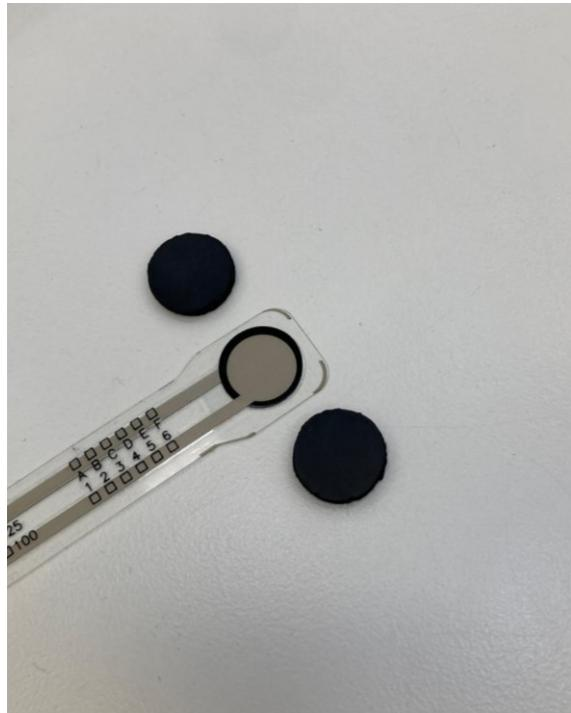
Figure 39. Flexiforce A201 FSR sensors and PU discs
