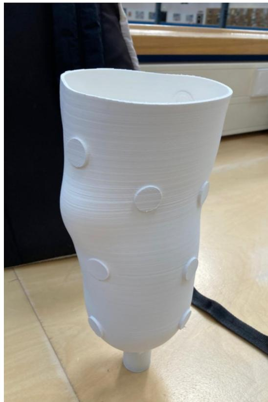
Figure 55. 3D printed realistic socket with spaces to locate FSRs.
