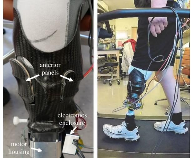
Figure 6. Automatic control of prosthetic socket size [25].
