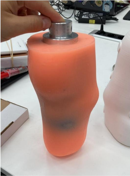
Figure 36. Realistic stump made from casted silicone, on top the adaptor to the machine can be seen. Inside of the stump there is a cement core.
