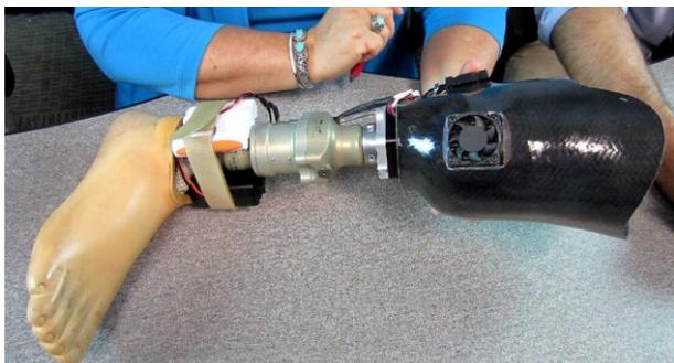
Figure 11. Aquilonix Prosthesis Cooling System by Leto Solutions [19].
