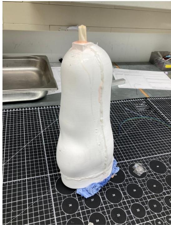
Figure 53. Realistic stump mould before demoulding.
