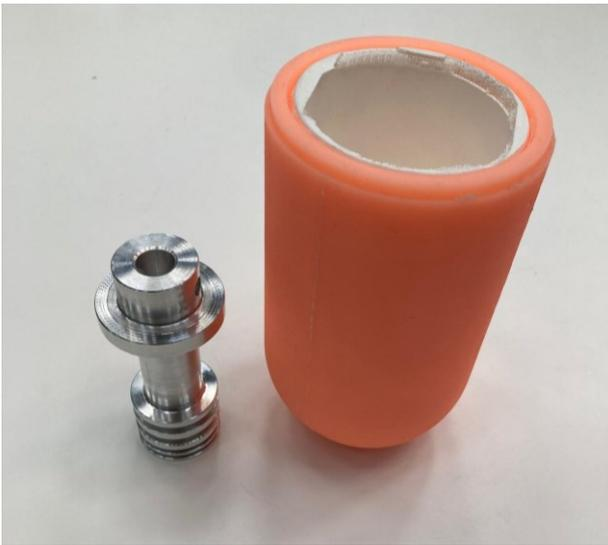
Figure 52. Here it is visible where the simplified stump part failed, on the left the aluminium fixture to connect the specimen to the cyclic loading machine is shown.
