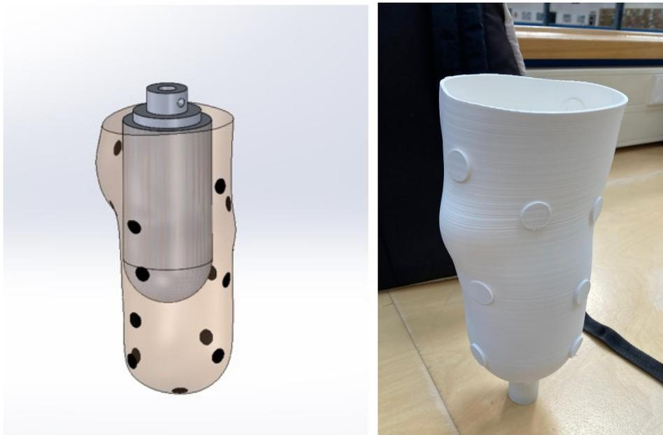
Figure 16. Realistic stump 3D model (left) and 3D printed socket (right)
