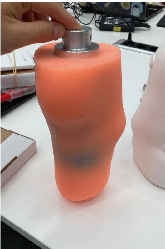
Figure 54. Demoulded realistic socket.
