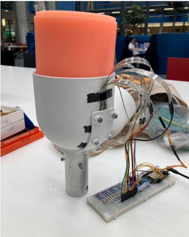
Figure 48. 3D printed prototype equipped and electronics circuit. Since this circuit uses a multiplexer, it just needs one resistor, so all those wires are not needed.
