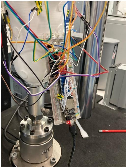
Figure 58. Close up view of the circuit and connections while the socket is fixed in the cyclic loading machine ready to be tested.
