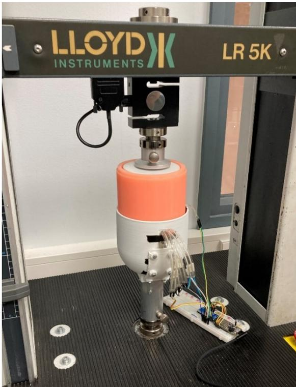
Figure 50. Prototype with integrated socket test
