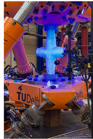
(b) Specimen placed in the TU Delft Hexapod
