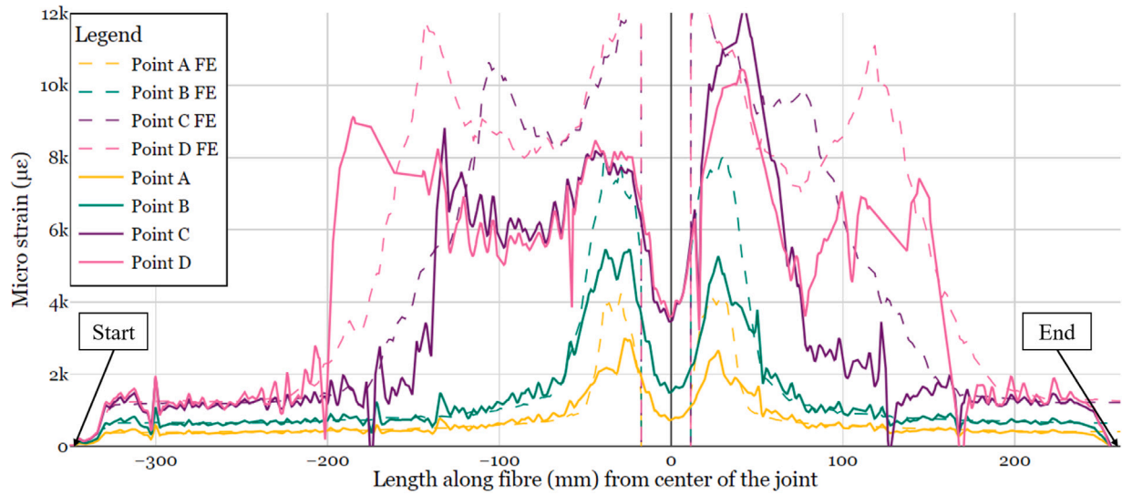
Fig. 8. Comparison optical fibre results experiment and FE model Nx-B26. With indication of start and end of optical fibre in Fig. 2(b).
