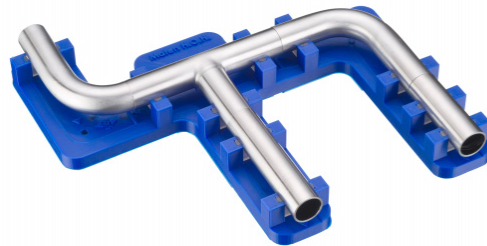
Figure 2.5.6: Support tool for welding parts
