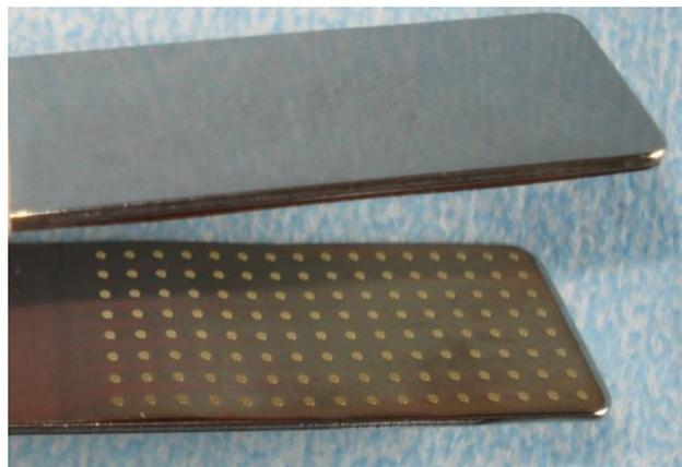
Figure 6 – Electrode arrays used for simultaneous endo-epicardial mapping
