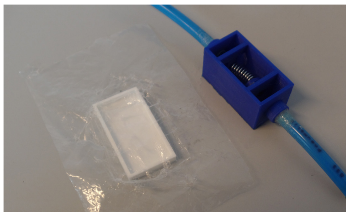
Figure 65: Form fit with plastic foil in between
