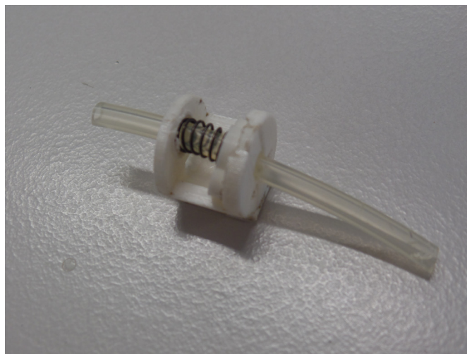
Figure 82: Parallel valve, silicone tube threaded through the spring
