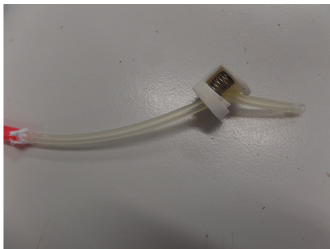
Figure 83: Parallel valve, silicone tube next to the spring. This enable the flexinol wires to thread through the spring.
