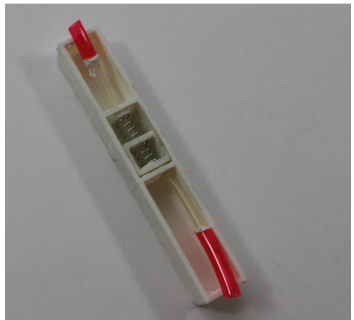
Figure 75: Concept parallel openend with two pair of sma wires in opposite direction. (SMA wires are missing in this photo)
