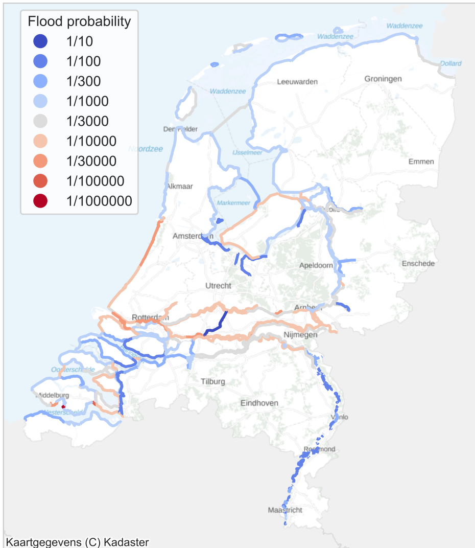
Figure 2.1.: Maximum allowable probabilities of flooding per year for flood defence segments in the Netherlands as described in the Water Act.
