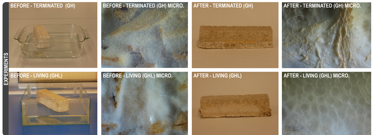
Figure 12: Experiments with long term water exposure (8 weeks) to terminated (above) and living (below) mycelium-based composites.
