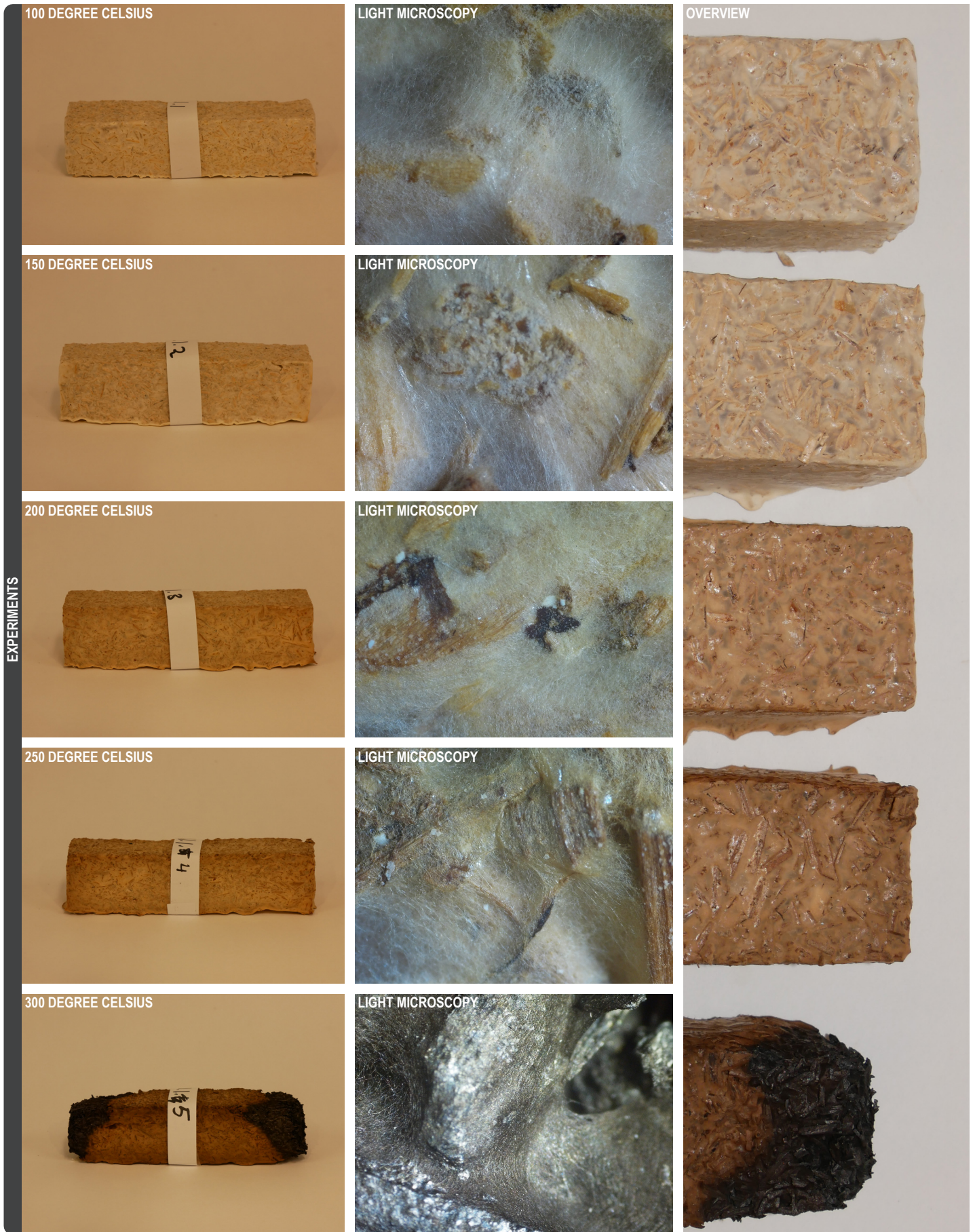
Figure 13: Experiments with 5 identical mycelium-based composites baked at 100°C, 150°C, 200°C, 250°C and 300°C (top to bottom).
