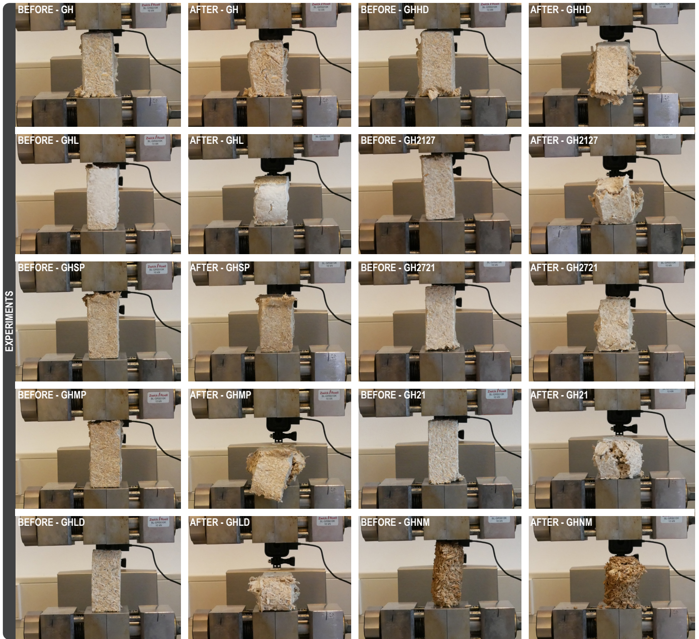
Figure 20: Before and after results of the compression test of various mycelium-based composites.
