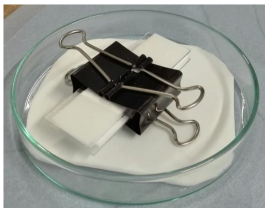
Supplementary Figure 2. Image of clamping system used to apply constant pressure.
